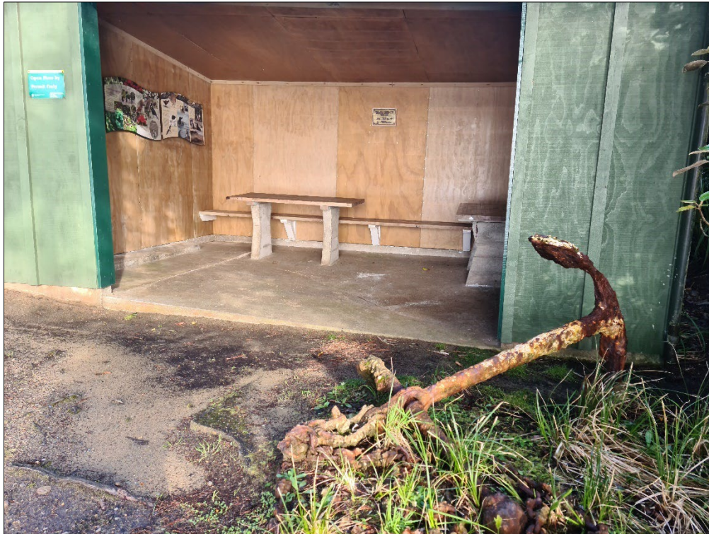
Figure 17: Bent-stock anchor outside the shelter at Sydney Cove, Ulva Island (Image: author).
