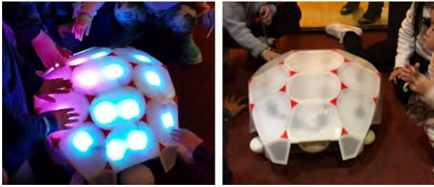
Fig. 1 When Shelly is “happy”, bright colors illuminate its shell [left]. When it’s “sad”, it hides its head and disables the lights for 14 s [right]. (Naver Labs). (Color figure online)
