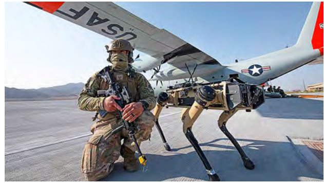
Fig. 3 The Ghost Vision 60 is a quadrupedal unmanned ground vehicle (Q-UGV) developed by Ghost robotics to carry out tasks such as remote inspection, intelligence, surveillance, reconnaissance, mapping, distributed communications, and persistent security
