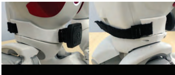
Fig. 2 [a] The customized NAO chest holder front side with the mobile magnetic holder. [b] is the holder back side with the added strap to fasten it.
