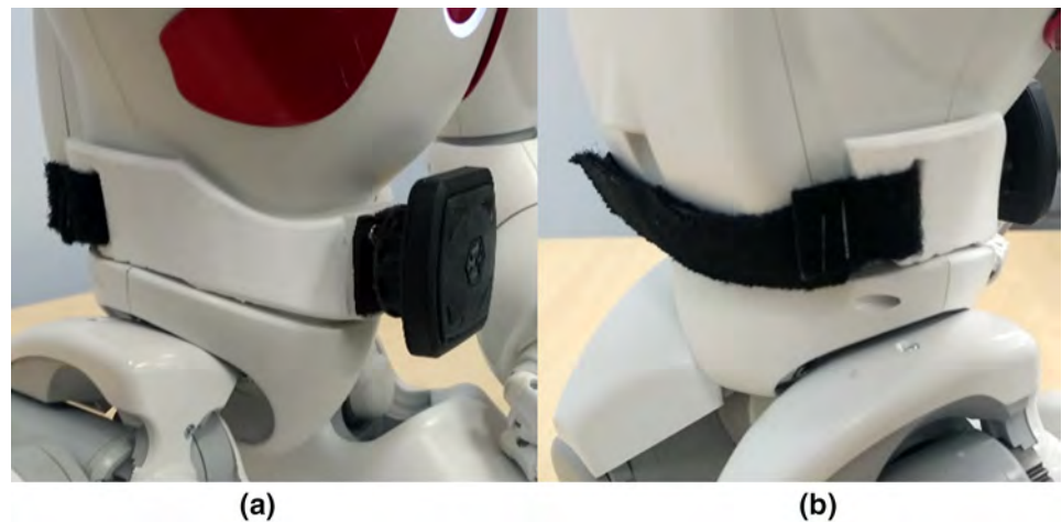
Fig. 2 a Custom-designed NAO chest holder side view, showing the attached standard mobile holder. b NAO chest holder rear view, showing the added Velcro strap for fastening
