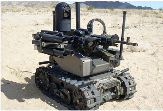
Fig. 1 The Modular Advanced Armed Robotic System (MAARS®) is an unmanned ground vehicle (UGV) developed by Qinetiq and designed for reconnaissance, surveillance, and target acquisition (RSTA) missions to increase the security of personnel manning forward locations
