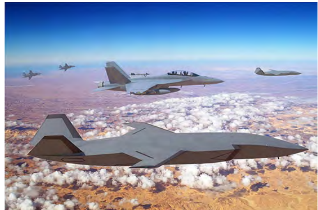
Fig. 4 Boeing Loyal Wingman is a low-cost stealth unmanned aerial vehicle (UAV) developed by Boeing Australia to support manned aircrafts such as the F-35 and perform autonomous missions using artificial intelligence. A squadron of Loyal Wingmen can be controlled by a parent aircraft to accomplish tasks such as scouting or absorbing enemy fire if attacked
