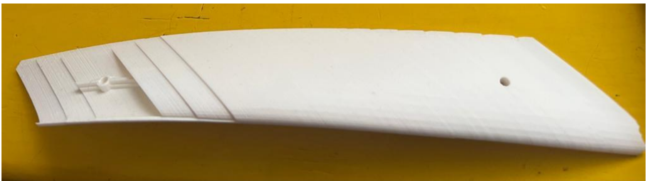
Figure 26: 3D printed Central Blade
