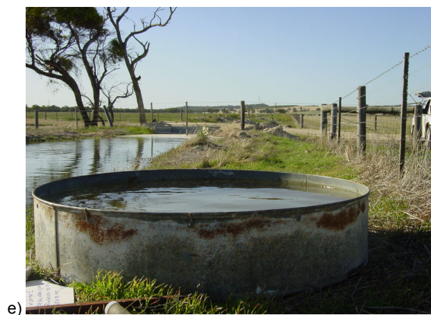
Plate 2. a) Instrumentation at NAP5, b) rain collection container for isotopic analysis, c) shaft encoder, d) sampling soil water from suction lysimeters post irrigation and e) Class A evaporation pan.
