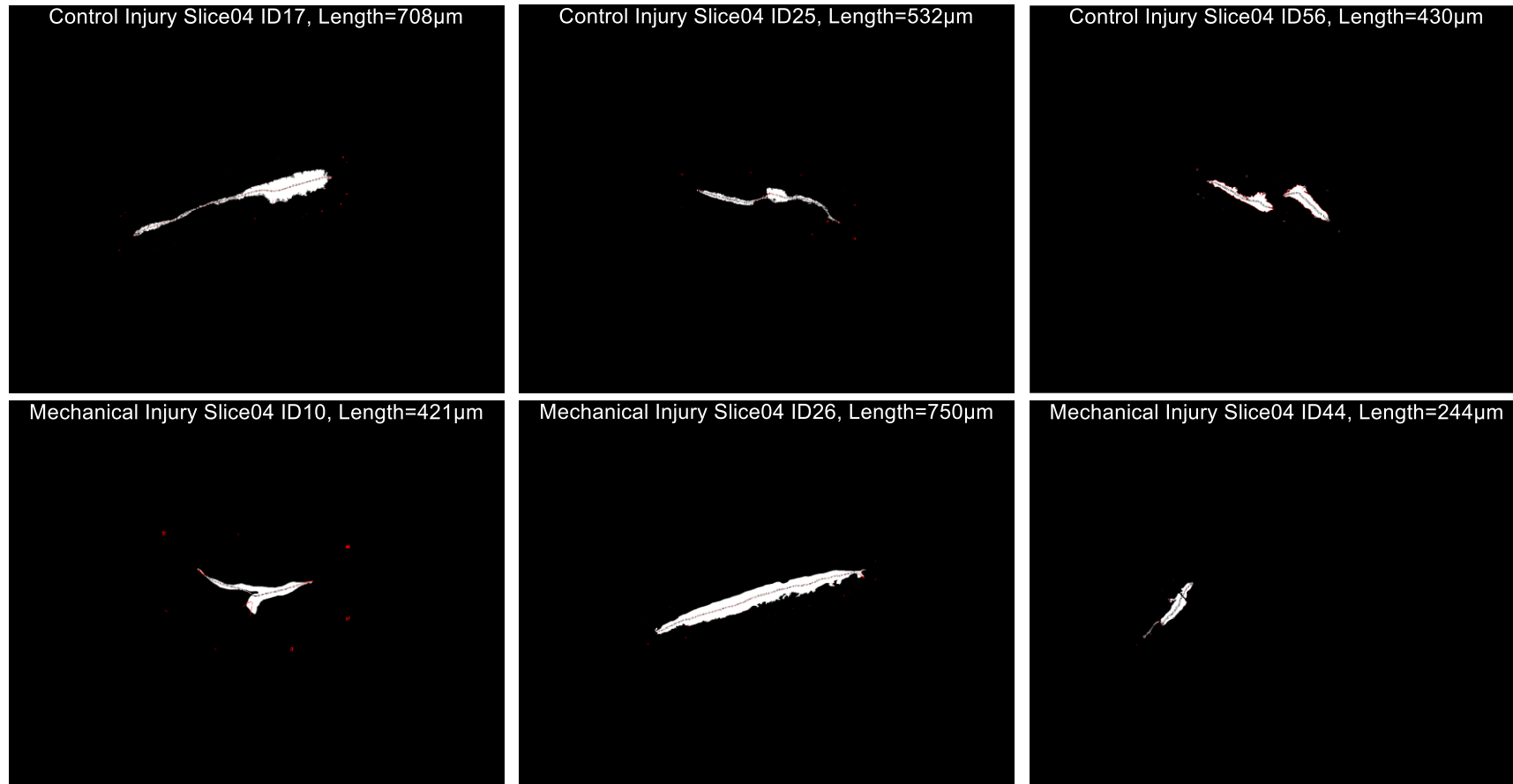
Figure C- 18 Length of needle injuries in slice 4. Each image is annotated with labels indicating control or mechanical injuries, along with the slice number and specific injury IDs, each with its respective length measurement. The top row displays control injuries, labelled as ID17, ID25, and ID56, respectively. The bottom row shows mechanical injuries, with labels ID10, ID26, and ID44, respectively.
