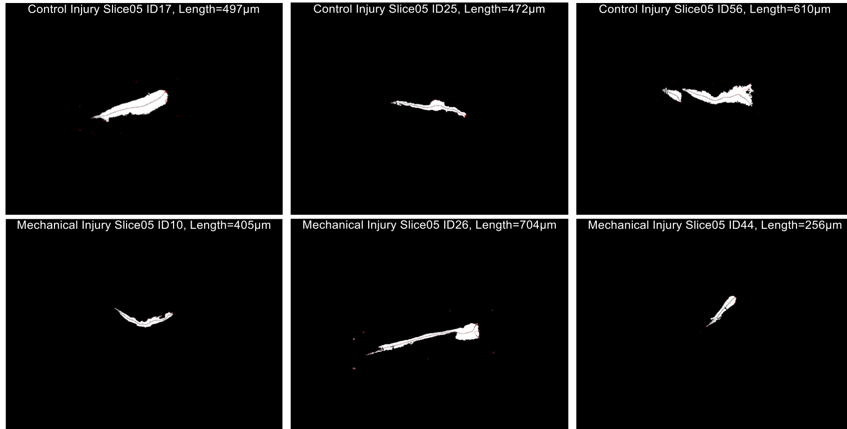
Figure C- 23 Length of needle injuries in slice 5. Each image is annotated with labels indicating control or mechanical injuries, along with the slice number and specific injury IDs, each with its respective length measurement. The top row displays control injuries, labelled as ID17, ID25, and ID56, respectively. The bottom row shows mechanical injuries, with labels ID10, ID26, and ID44, respectively.
