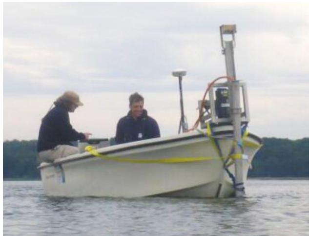
*Figure 17: Image of Innomar SES-2000 subbottom mounted on the bow of the vessel with Seatex MRU (Photo: J. Benjamin).*
