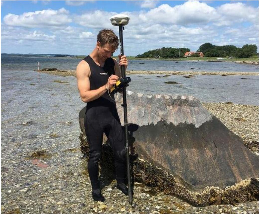
Figure 15: Collection of site locations at low tide with a Trimble R8 RTK (Photo: J. Benjamin).
