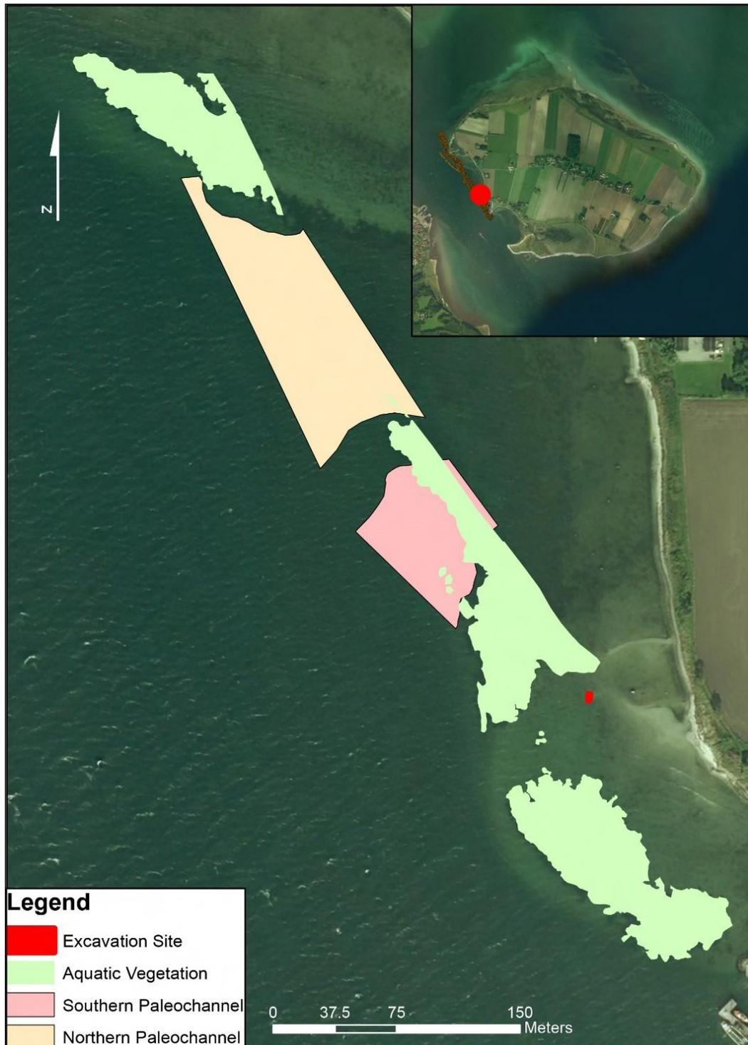
Figure 37: Aerial imagery of digitized aquatic vegetation and paleochannels using the sidescan sonar and subbottom profiler. The representations depict the extents of the sonar data.
