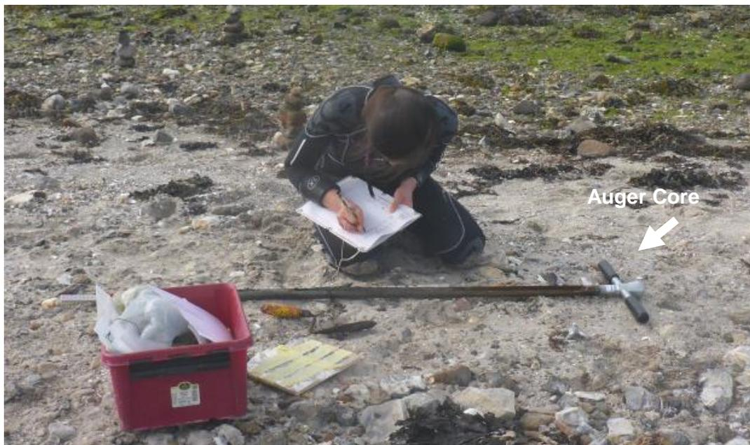
Figure 23: Geotechnical sample logging through the use of an auger corer (photo: J. Benjamin).
