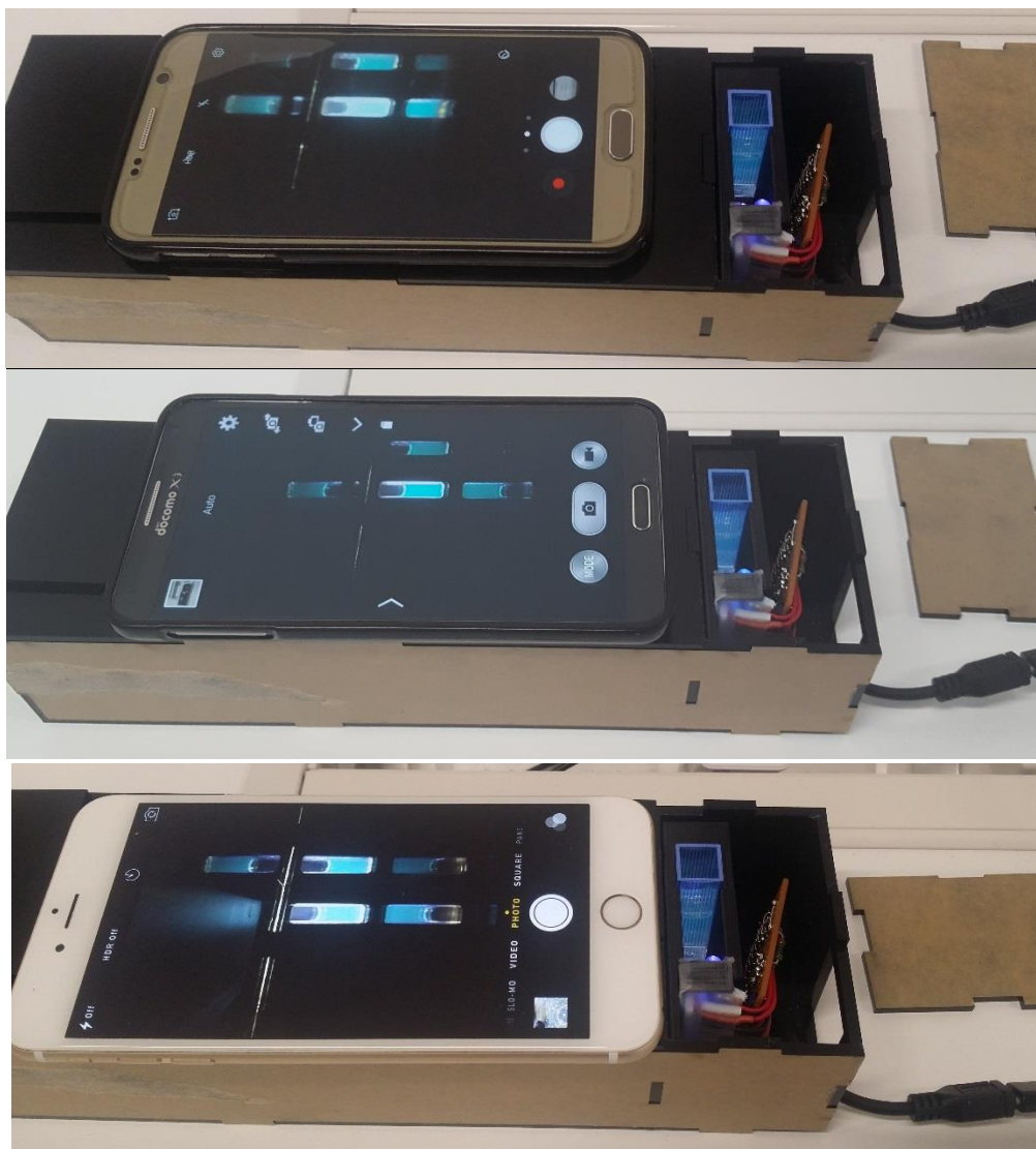
Figure 25: The device was working with Samsung S7, Samsung Note 3 and Iphone 6, respectively. (The small lid is left opening to show the light source and the cuvette's position. In the tests, this lid will be closed completely).
