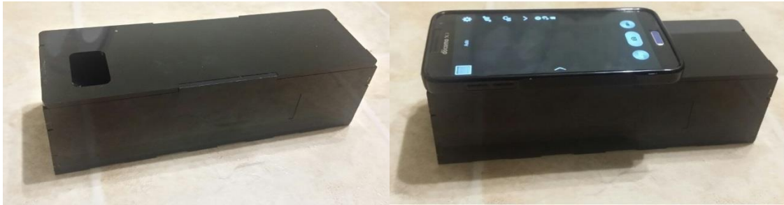
Figure 13: The black box design for smartphone based device to detect and quantitate HSA level in urine.
