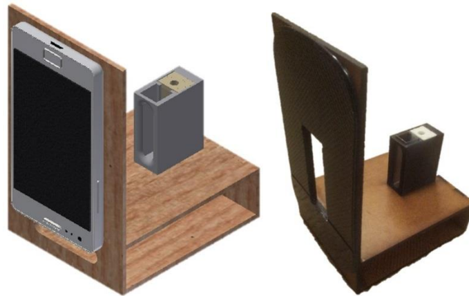
Figure 12: The design using LED to supply the UV light for exciting the mixture of BSPOTPE and HSA in urine (Keen et.al 2016).
