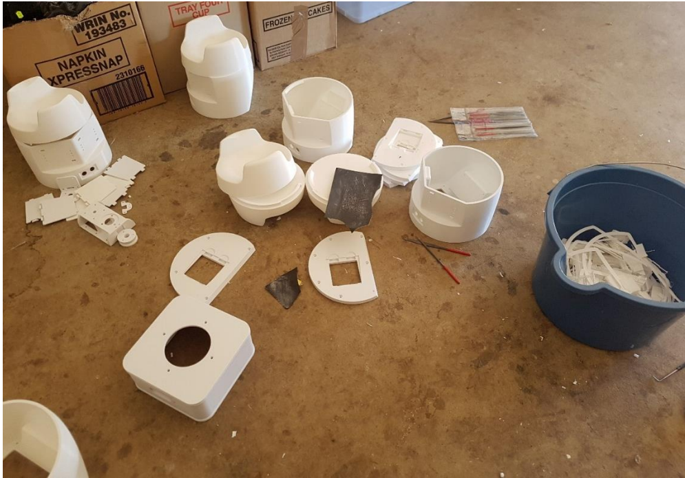
Figure 118: Preparing the 3D printed parts for painting by through removal of supports and sanding
