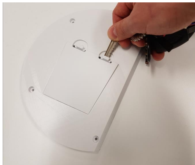
Figure 97: A simple set of keys can unhinge the snap-fit cover
