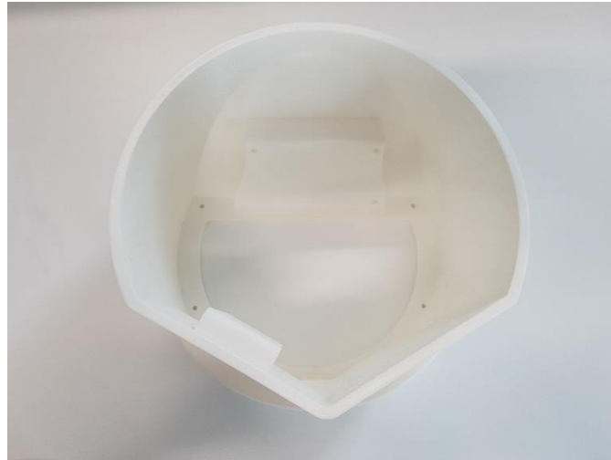
Figure 76: Top view of the preliminary marker enclosure 3D print showing no top half provides improved accessibility for electronic mounting
