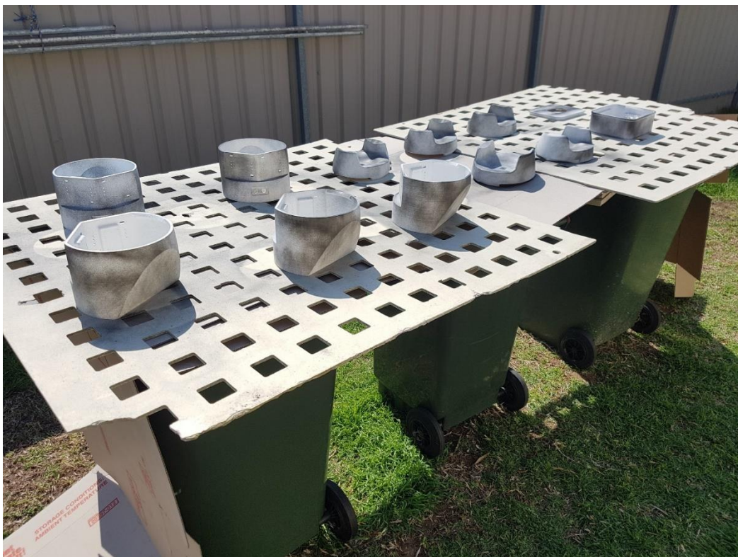
Figure 119: Painting set-up and application of initial light coat
