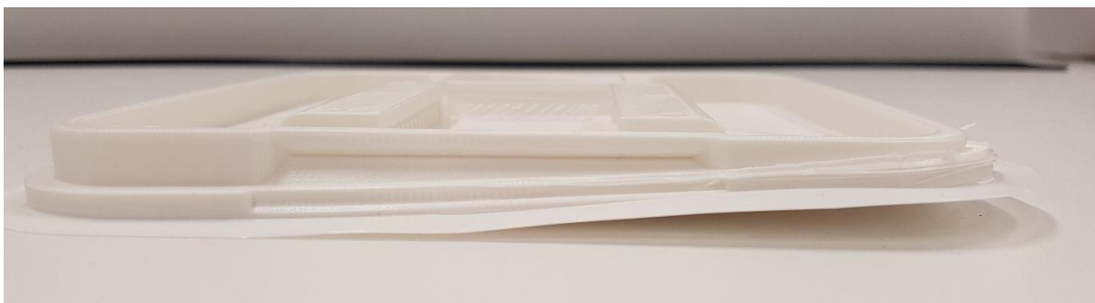
Figure 143: 3D printing failure for the master enclosure base
