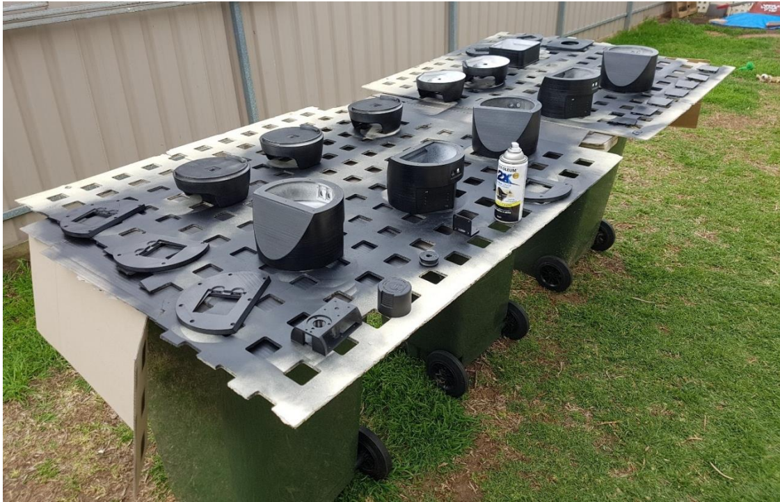
Figure 120: Progressive painting of the enclosures
