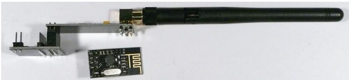
Figure 124: Current nRF24L01+ module (bottom) compared against a high powered module (top) (Tangient LLC, 2018)
