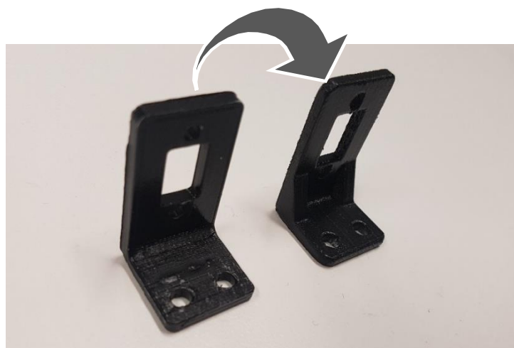
Figure 141: Transmissive photo-interrupter mount design optimisation
