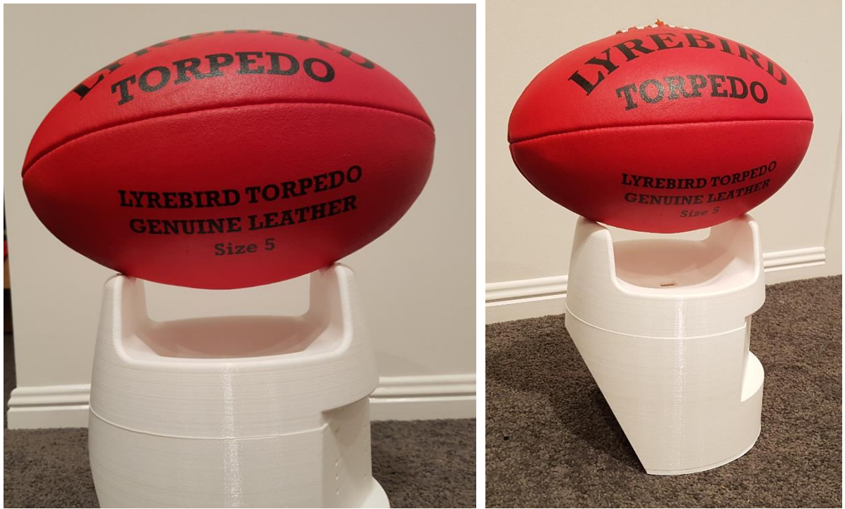
Figure 80: Testing the preliminary marker enclosure with an Australian football
