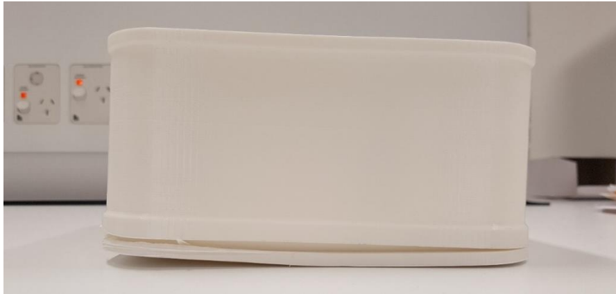
Figure 144: 3D printing failure for the master enclosure
