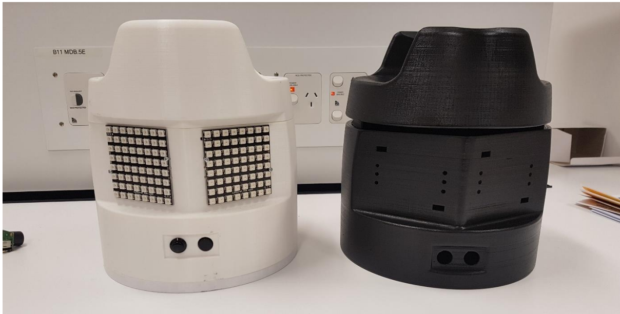
Figure 122: Comparison of a black painted slave enclosure next to an unpainted white one
