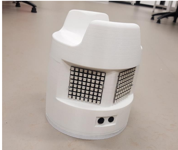
Figure 85: Mounting the LED matrix to the marker enclosure
