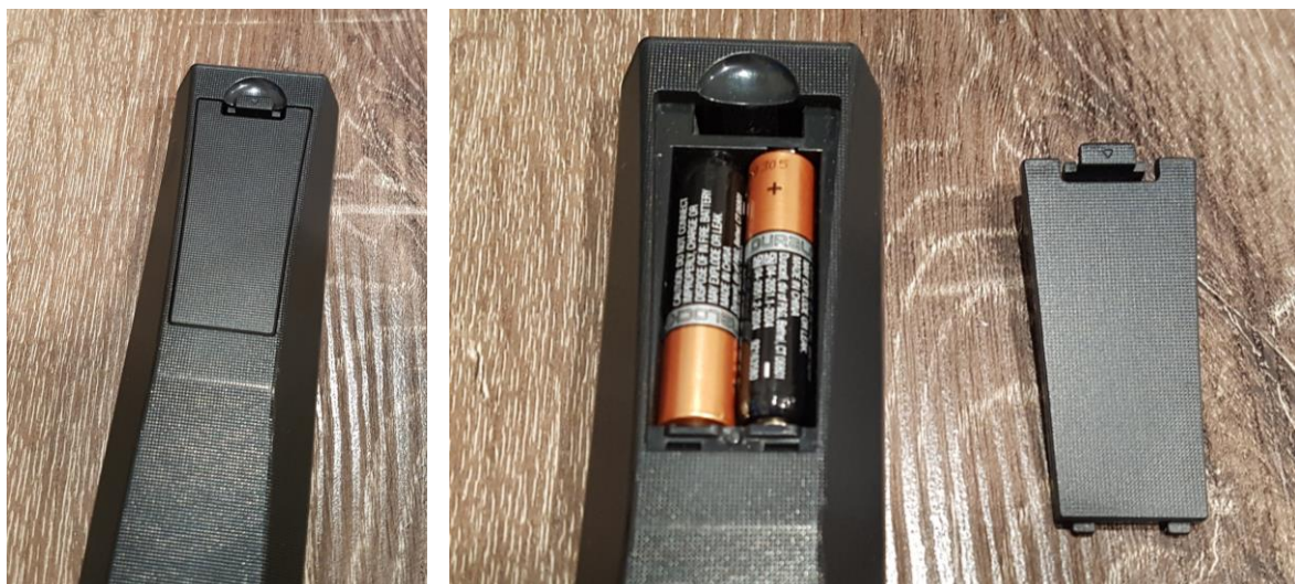
Figure 65: Inspiration from a simple TV remote for developing a snap-fit case
