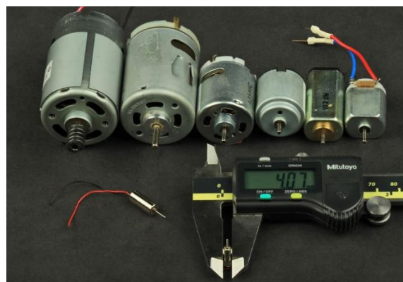
Figure 46: Various types of DC motors (Earl, 2015)
