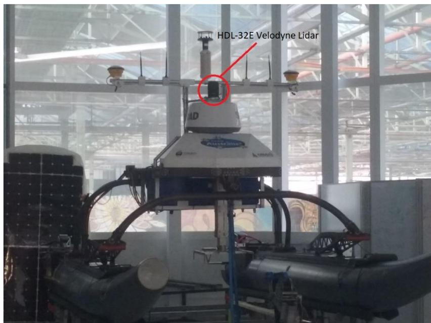
Figure 5. Location of the HDL-32E Velodyne lidar on the TopCat
