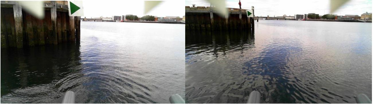
Figure 11. USV vision of the rotated green triangle from different approach angles
