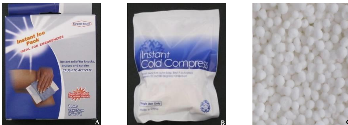
Figure 1-10: Images of Instant cold pack which contains loose AN prills and a water capsule (A&B) and prills of AN obtained (C).
