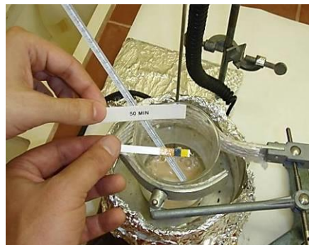
Continued release of ammonia after 50 minutes
