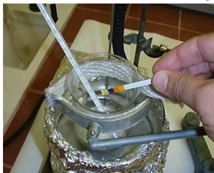
Release of ammonia after 1-2 minutes (over ≈ 110°C)
