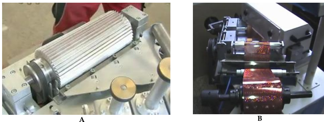
Figure 6-3: Glitter manufacturing process. A) Close-up of the rotary blade and a stationary bed knife. B) Metallised plastic film being fed into the cutting blade
