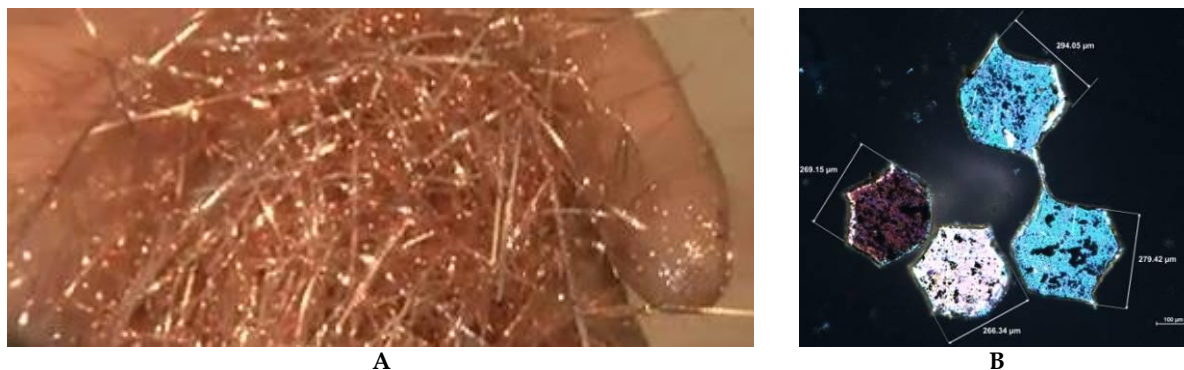
Figure 6-4: Glitter imperfections. A) Formation of “glitter grass”. B) Tears, poor cuts and unsymmetrical glitter
