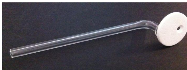
Figure 2-6. Picture of a film holder used in the NICISS foam film experiments.
