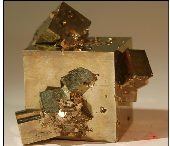
Figure 1.2 Image of unoxidised pyrite. A museum sample of pyrite showing negligible oxidation [17].
