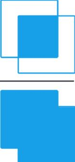
Figure 4.4: IoU Illustration (“Intersection over Union (IoU) for object detection - PyImageSearch,” 2020)
