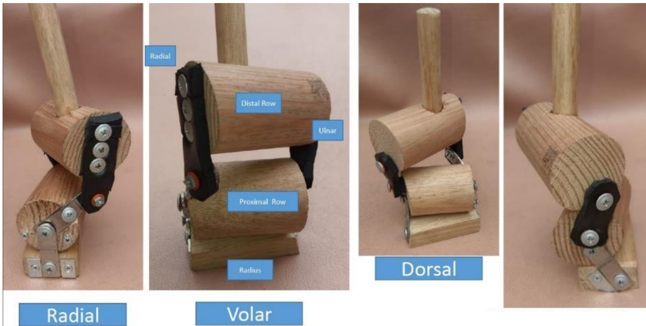
Figure 20. Wakefield Carpal Model - Model of the wrist as a series of single axle cylinders to allow adequate flexion and extension range.
