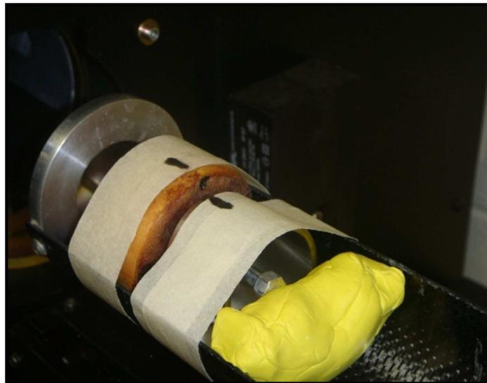
Femoral head and screw construct undergoing micro-CT scan to test different scanning protocols to achieve the optimum image quality
