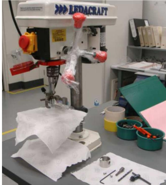
Figure 5.7: A commercial bench-top drill press was used for drilling the pilot hole and performing initial screw insertion prior to head contact.
