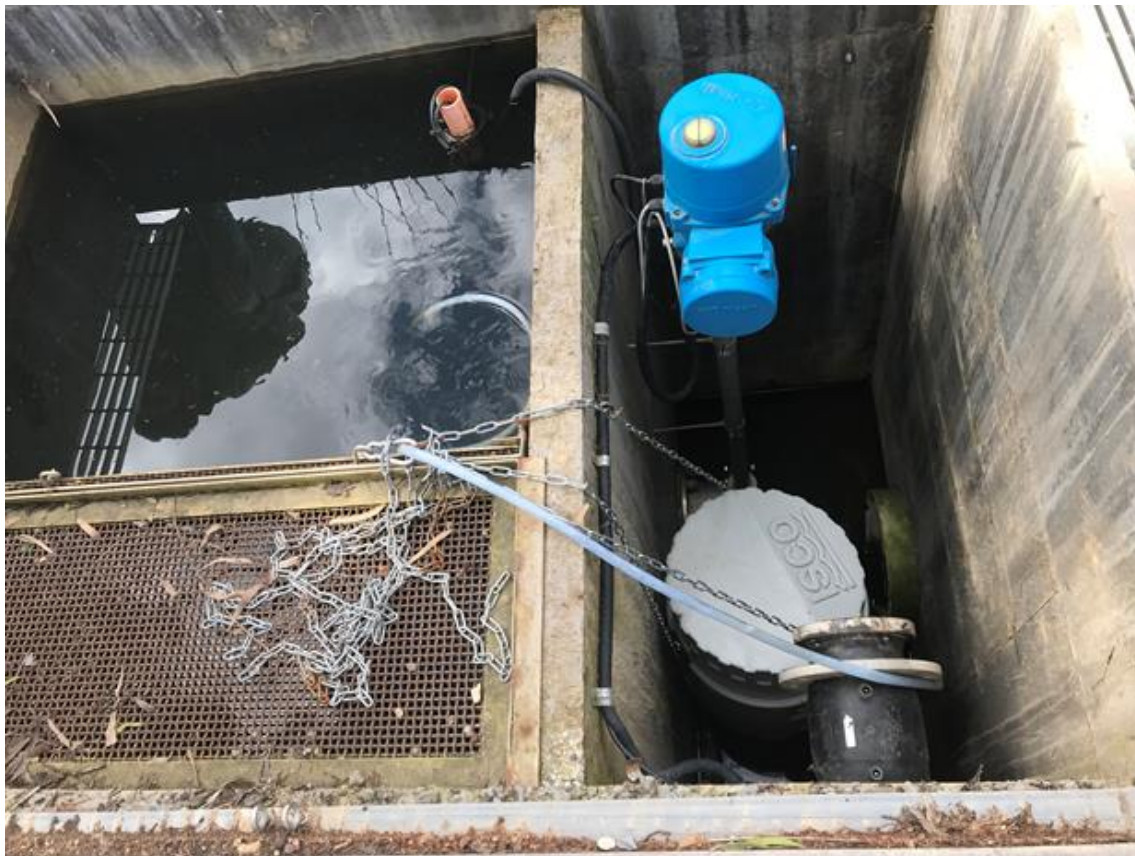
Figure 2. 5 Auto Sampler installed in Outlet pit of Oaklands Park wetland to collect composite samples to capture storm events from July 20 2018 to Sep 3, 2018
