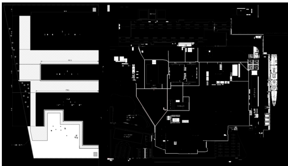
Figure 31 Failed attempt at creating binary occupancy grid for shipyard
