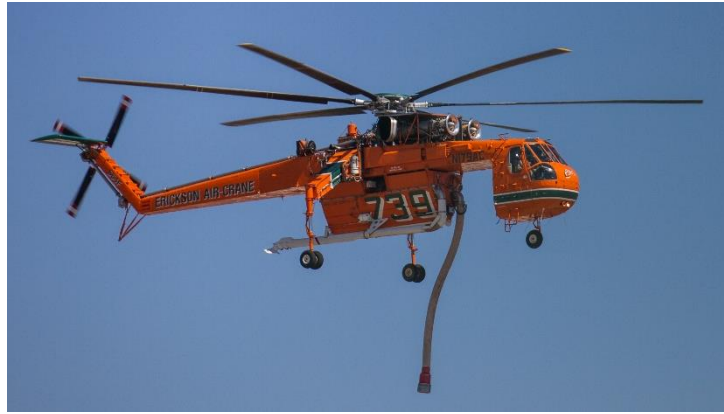
Figure 1-2: Erickson Aircrane with refilling snorkel suspended [7].
