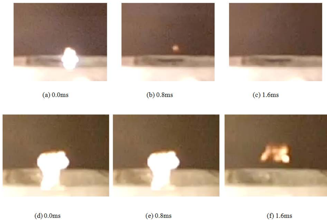
Figure 6.19: High speed camera frames of the laser initiation of a MWCNT surface (a-c) and the same sample with a layer of PETN (d-f).
