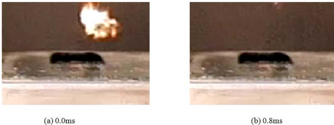
Figure 6.25: High speed camera frames of MWCNT (~2mm) array initiated by laser. Only one frame of flame is observed and very little ablation of particles can be seen.
