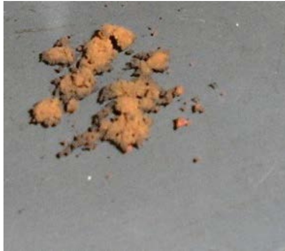
Figure 5.2: Photograph of iron nanoparticles (26nm) after camera flash unit initiation displaying an orange colour due to oxidation. (Reproduced from Chapter 3.2)
