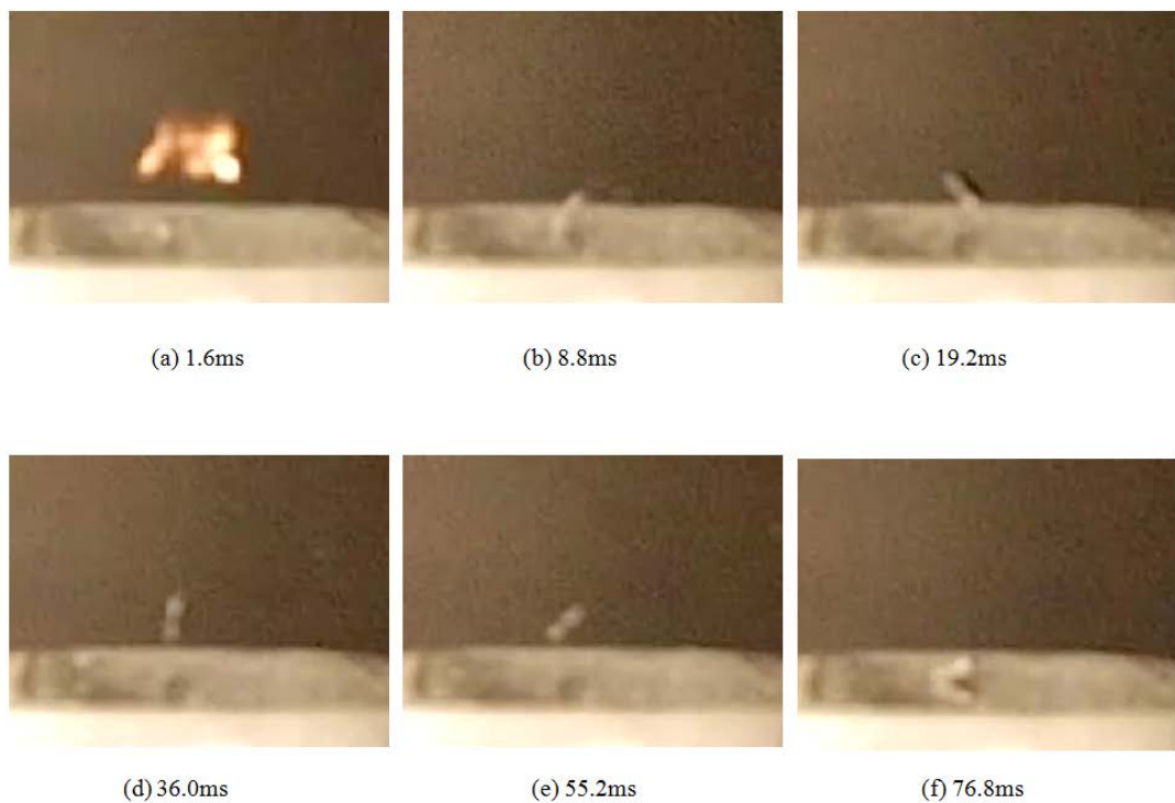
Figure 6.20: High speed camera photos of the MWCNT surface with PETN layer displaying the silicon wafer flipping through the air.
