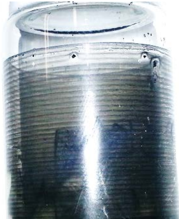
Figure 5.9: Horizontally aligned rows of carbon nanotubes on glass produced by the 'coffee cup effect' during evaporation.
