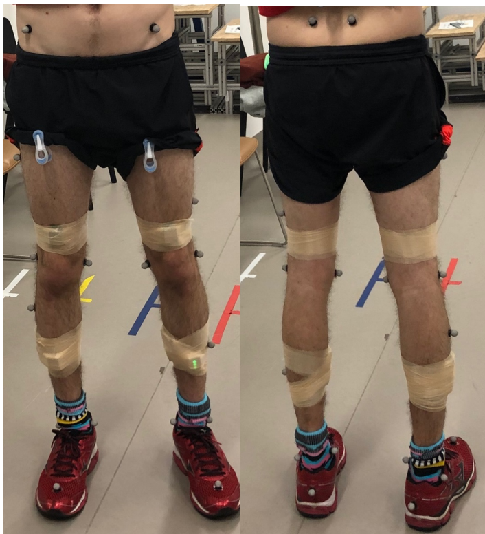
Figure 11: Participant lower body mark-up with Vicon reflective markers, 6 Delsys sensors and 2 SensorTags (Lateral Shank: right leg, Medial shank: left leg)
