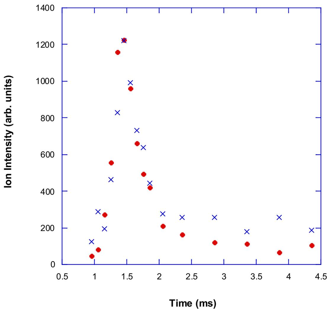
Figure A.2.2: Graph of the intensity of allene molecules (•) and propargyl radicals (×) detected in the TOFMS, as a function of time from the pulser fire. The intensity of propargyl radicals has been multiplied by 624 for clarity.
