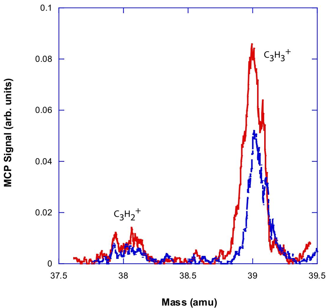
Figure A.2.3: TOF spectrum of the photofragments of allene, at excimer laser powers of 20 mJ/pulse (solid curve) and 60 mJ/pulse (dashed curve).
