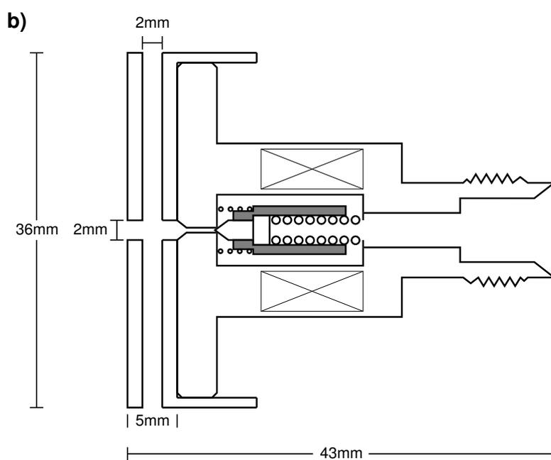
Figure A.1.1: Pictorial representation (a) and schematic diagram (b) of the pulsed nozzle with the thermalisation adaptor fitted.
