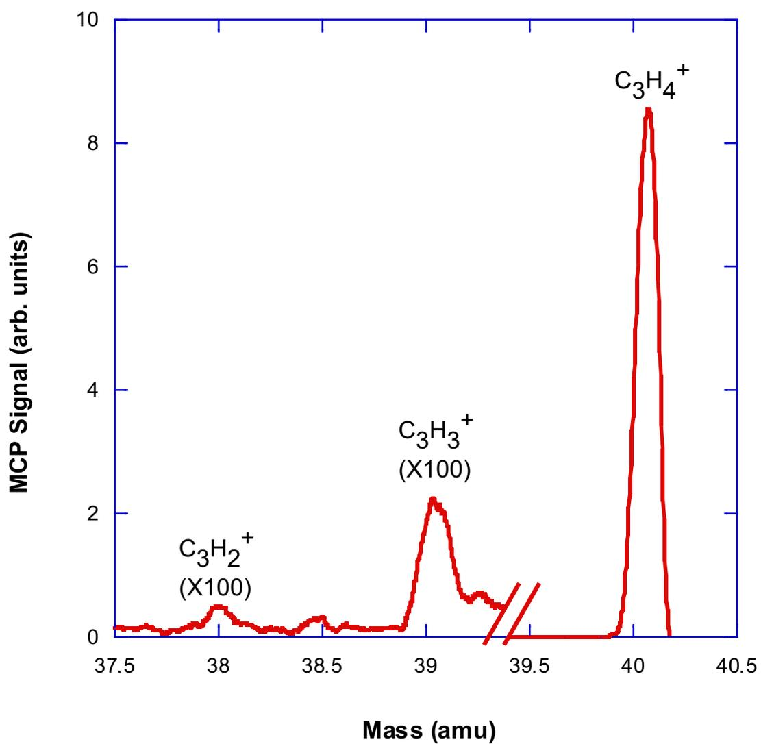
Figure A.2.1: A typical TOF spectrum of the photofragments of allene and the allene precursor. The signal of the photofragments has been multiplied by 100.
