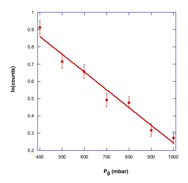
Figure 3.2.4: A typical result for Beers attenuation, shown here in the 120° elastic scattering of electrons from Ar. The error bars represent the variation in the electron counts due to statistical and pulse-by-pulse density variations.
