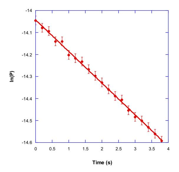
Figure 3.2.2: A plot showing the natural log of the collision chamber pressure, P, (•) as a function of time, once the pulsed nozzle was closed. A linear function has been fitted to the data. The error bars represent the gauge resolution.
