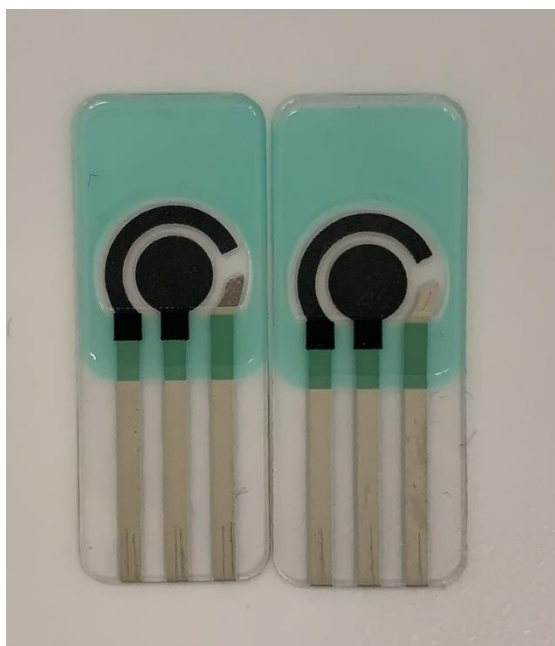
Figure 3 Comparison of modified and unmodified reference electrode
