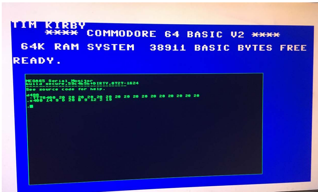
Figure 23. Matrix Mode, memory read and write
