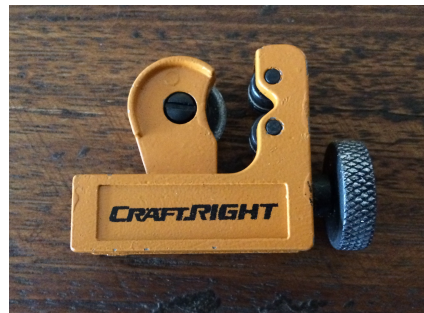
Figure 3-2 - Rod cutter used to customise the flexible intramedullary nails
