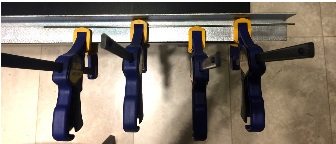
Figure 3-4 - Setup of steel offcut and flexible intramedullary nail to bend the nail tip
