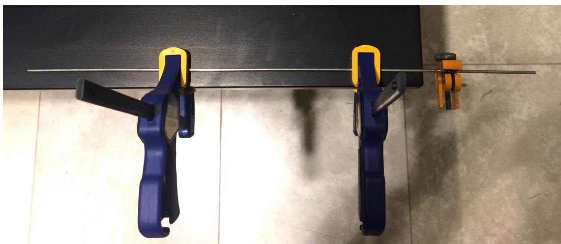
Figure 3-3 - Cutting flexible intramedullary nail setup
