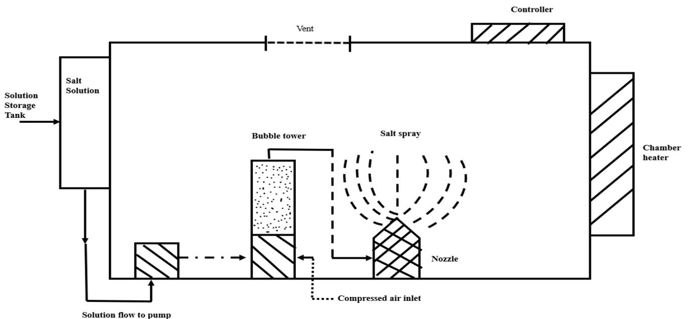
**Figure 3.4** Schematic diagram of cyclic corrosion chamber
