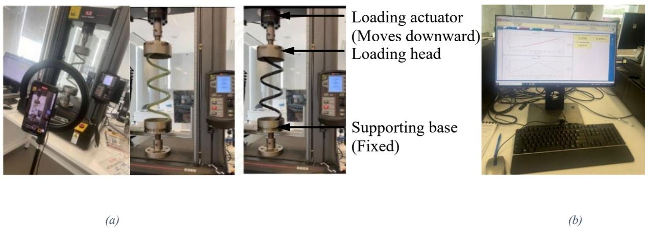
**Figure 3.3** (a) Installation of composite helical springs (GFRP and GCFRP) into a universal testing machine for applying compression load and (b) data recorded directly from the INSTRON 5969
