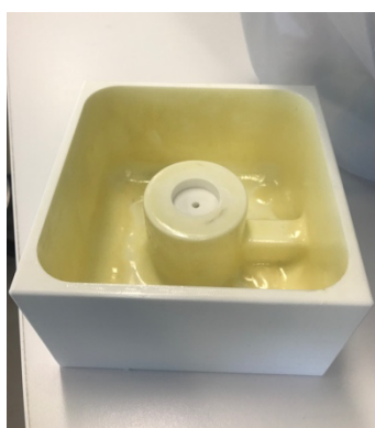
Figure 5: Electrochemical chamber for polarization tests
