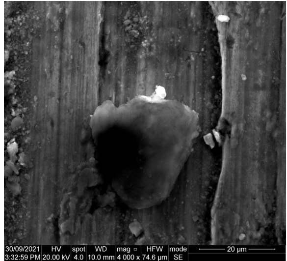
Figure 18: SEM images for worn surface at 992.1 MPa and 5 mm sliding distance with Ti-6Al-4V on the left and Ti-6Al-7Nb on the right
