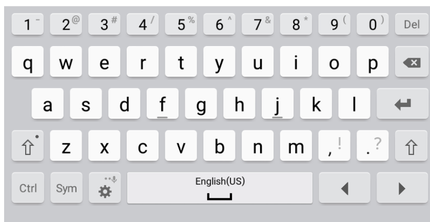
Figure 5.1: A representation of the Software keyboard on a Samsung Galaxy tablet, as presented in portrait mode. Key activation is touch based with additional keyboard symbols accessed through the "Sym" button.
