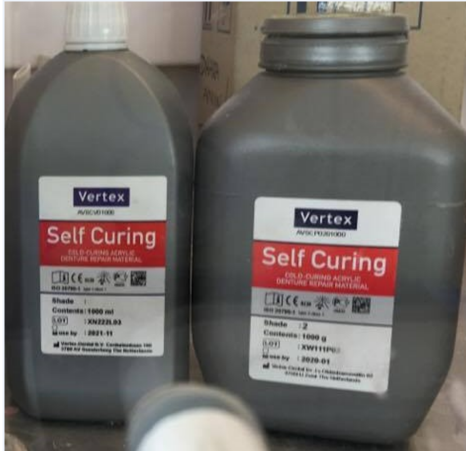
Figure 7: Acrylic powder and liquid used to make PMMA
