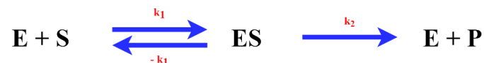
Figure 11 – Schematic representation of an enzyme mediated reaction where k_1 is the rate of ES complex formation, -k_{-1} is the rate of ES dissociation reverse to enzyme and substrate, and k_2 is the rate of ES dissociation resulting in product (P) formation. The overall rate of reaction is restricted by the amount of available free enzyme and by the degradation of the ES complex.
