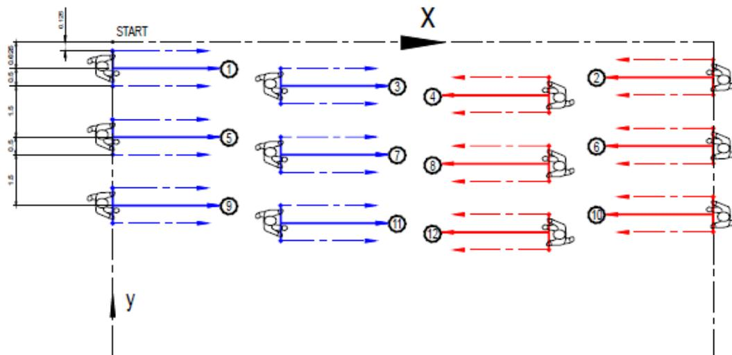
Figure 20: Grid configuration when instrument was set to grid mode to get maximum resolution – diagram is illustrating data acquisition at 4 lines per meter (0.25m spacing) and in zig zag configuration (Bartington 2012).
