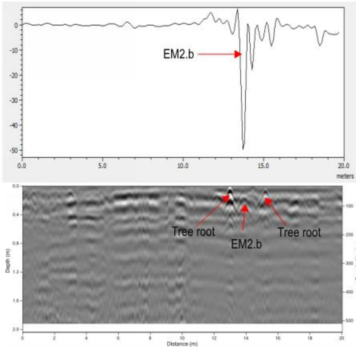
Figure 64: GPR profile 13 and corresponding 2D magnetics profile their alignment and location is depicted in Figure 61 by the green arrow from E (0) to F(20).
