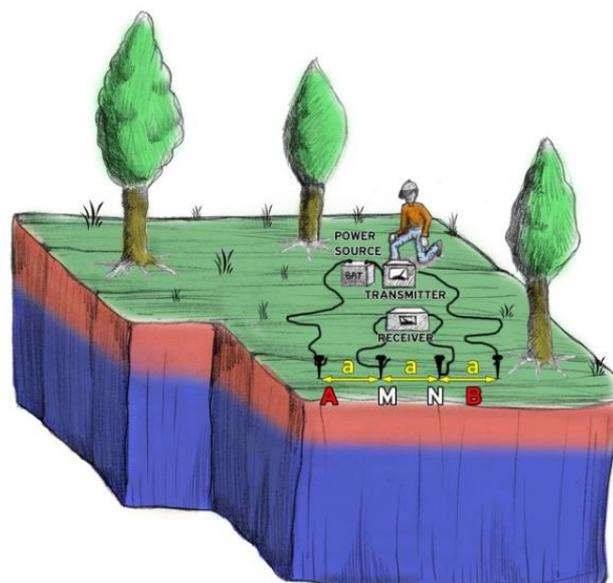
Figure 24: The Wenner array survey configuration,  $a$  = electrode spacing,  $A + B$  = current electrodes,  $M + N$  = potential electrodes. The four electrodes A, M, N and B are equally spaced along a straight line (diagram created by Kleanthis Simyrdanis).
