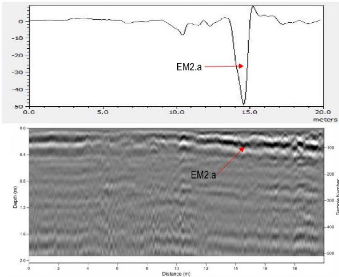
Figure 62: GPR profile 69 and corresponding 2D magnetics profile their alignment and location is depicted in Figure 61 by the red arrow from A (0) to B(20m).
