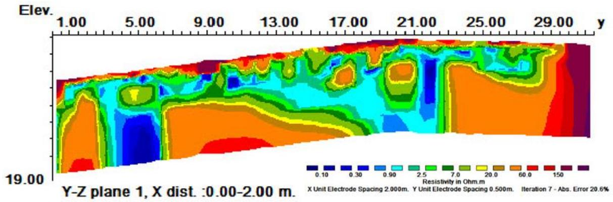
Figure 68: The first pseudo-section constructed from line one (beginning) of the dipole dipole array electrode line.
