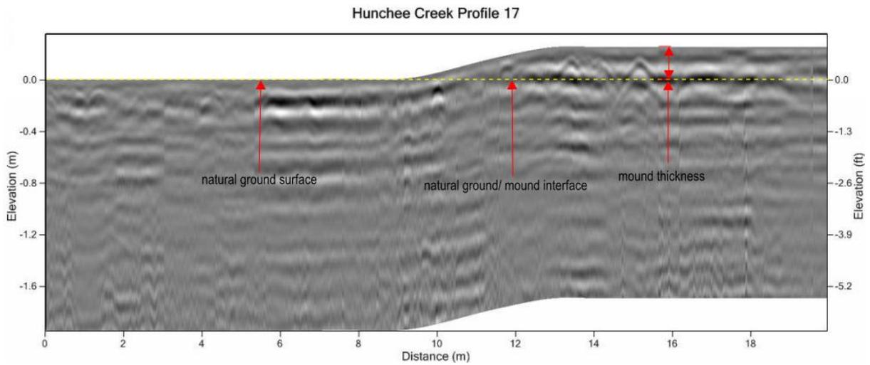
Figure 58: 2D GPR profile 17 topographically corrected and annotated, mound extents and depth were derived from all other profiles in this manner.
