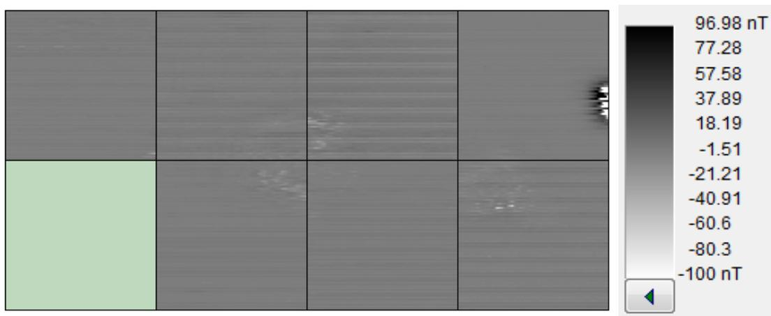
*Figure 27: Seven combined magnetics datasets, processing was required to remove the stripes and also the high responses from the stormwater pipe in the top right grid square.*
