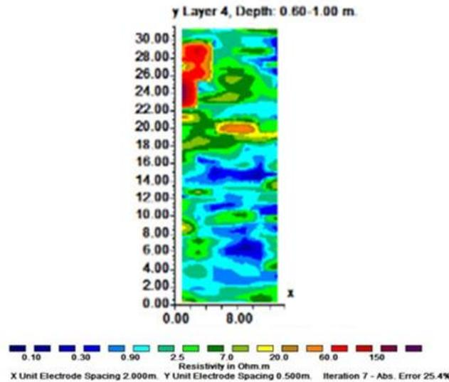
*Figure 31: An example of a 3D inversion slice from the Wenner Array dataset collected over one of the mounds, resistivity is expressed in ohms per metre in a colour scale below the dataset. The depth of the slice has been take from 0.6m to 1.0m.*
