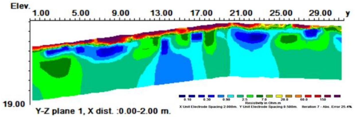
Figure 71: Wenner Array – pseudo-section of electrode line 1, the first line of the survey grid.
