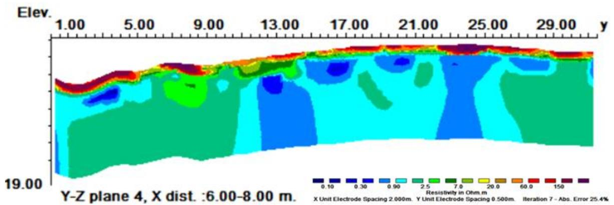
Figure 72: Wenner array pseudo-section, electrode line 4, the centre line of the survey grid.
