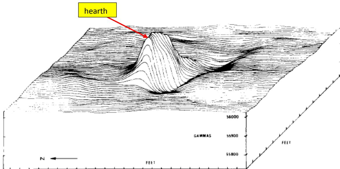
*Figure 6: An isometric presentation of the total magnetic field plotted 0.5m above a camp fire hearth created by Stanley and Green as a test case. The data set is in gammas which is an older order of measurement to nano-tesla, however 1 gamma = 1 nano-tesla. Remanent magnetism parallel to the Earth's field was induced in the ferromagnetic minerals in the soil beneath the fire (From Stanley and Green 1976:56).*
