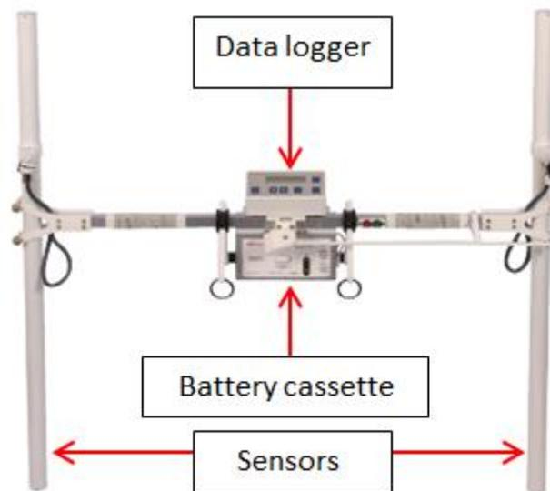
*Figure 19: Bartington Grad601 – Dual Sensor Gradiometer (Bartington 2012).*
