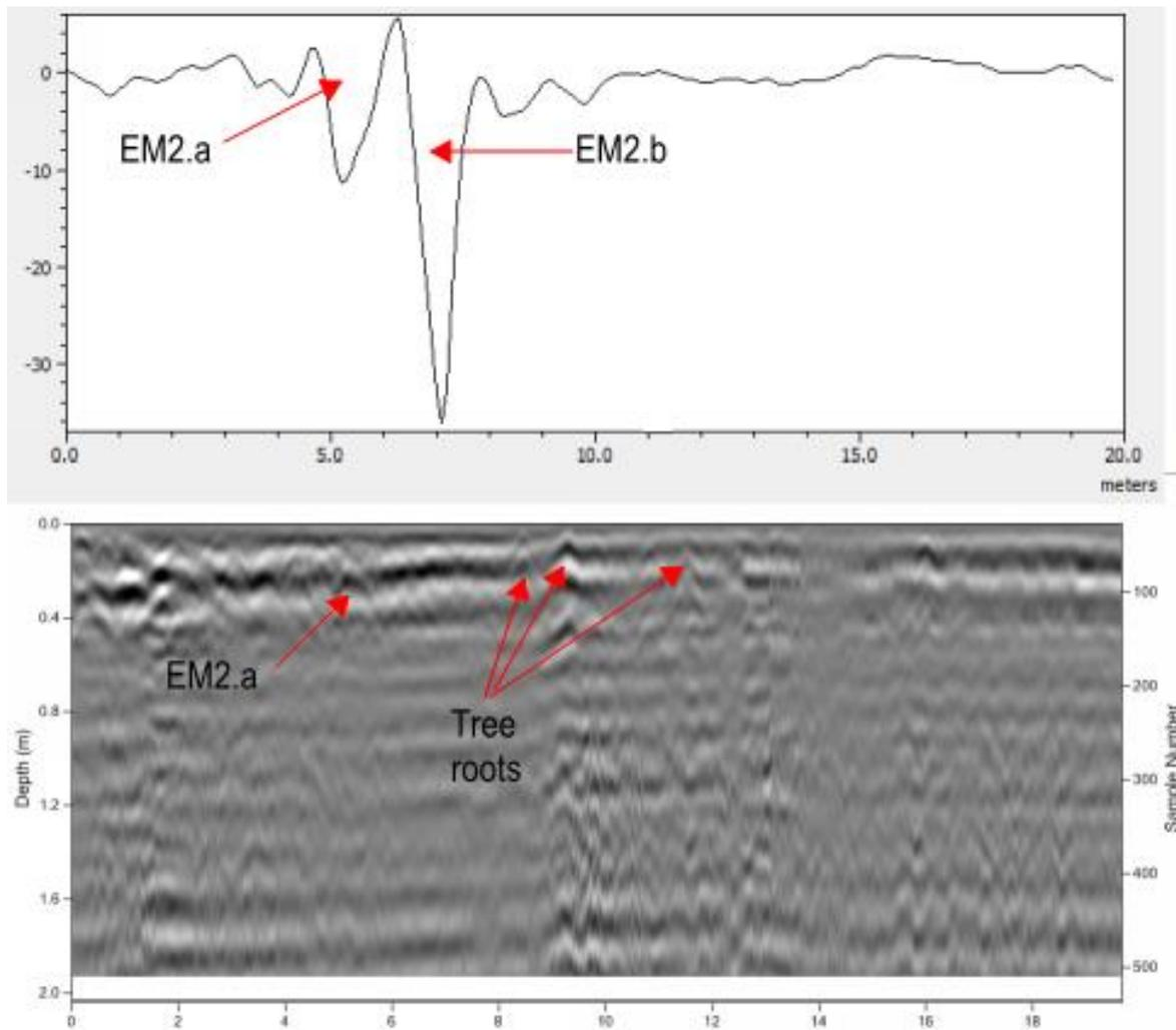
Figure 65: GPR profile 70 and corresponding 2D magnetics profile their alignment and location is depicted in Figure 61 by the blue arrow from G (0) to H (20m). EM2.a has been detected again in both the magnetics and GPR profiles. EM2.b has not been detected in the GPR profile.
