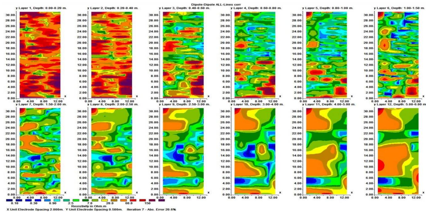
Above: ERT (Electrical Resistivity Tomography) Dipole-dipole Array formulated from lines 1-7
