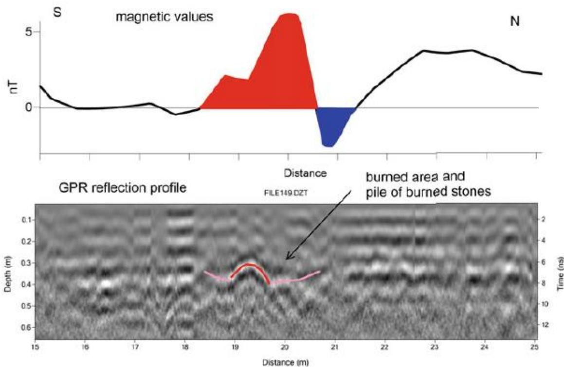
Figure 13: Combined 2D GPR profile and 2D magnetics profile interpretation approach, the dataset indicates a burned area with a pile of stones from an earth oven (Conyers 2018:99).
