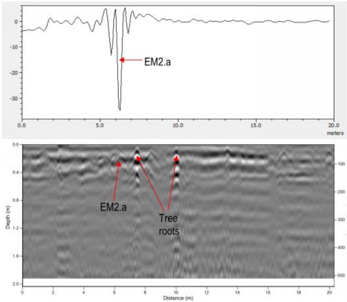
Figure 63: GPR profile 10 and corresponding 2D magnetics profile their alignment and location is depicted in Figure 61 by the yellow arrow from C (0) to D(20)m.
