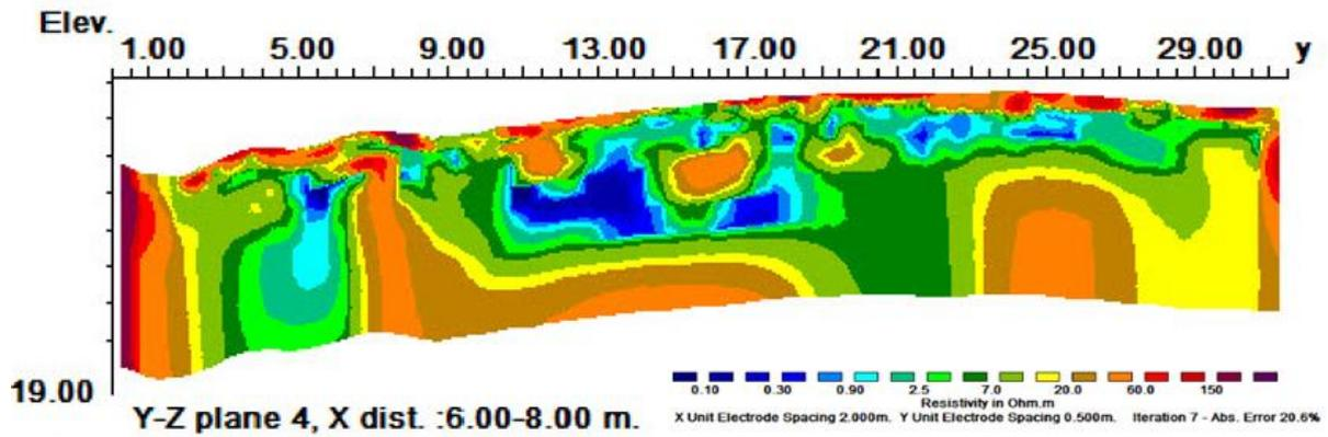
Figure 69: Dipole-dipole pseudo-section from the middle of the survey grid, electrode line 4.
