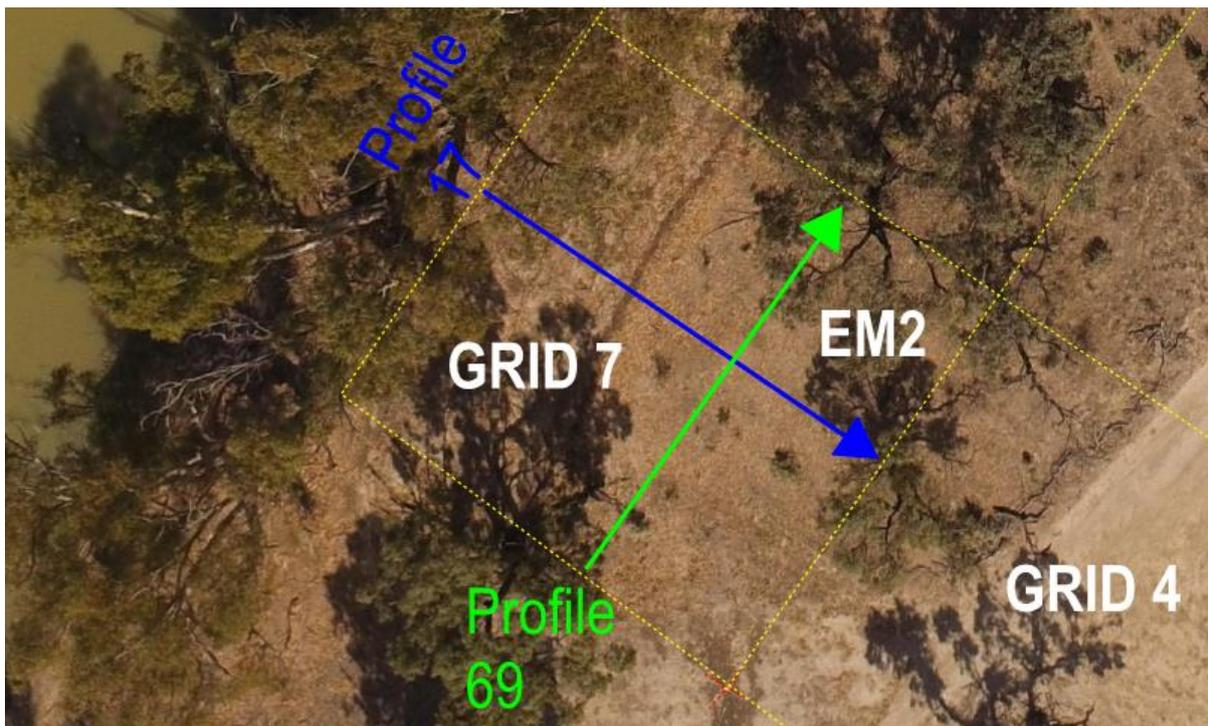
*Figure 56: Map showing the alignment of profiles 17 and 69, eighty 2D profiles from both x and y axis were analysed and extents and depth tabulated in order to delineate the mound extents and mean depth.*
