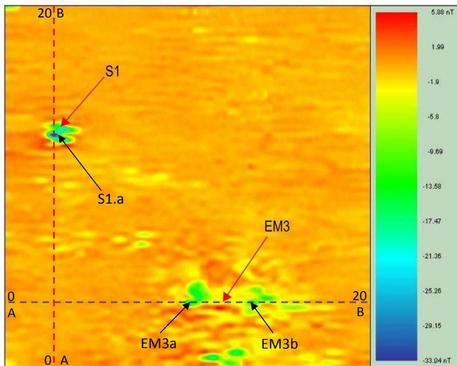
Figure 50: is the 20m x 20m magnetic dataset of grid eight the colours within the dataset coincide with colour scale to the right of the dataset; readings are expressed in nano-tesla.
