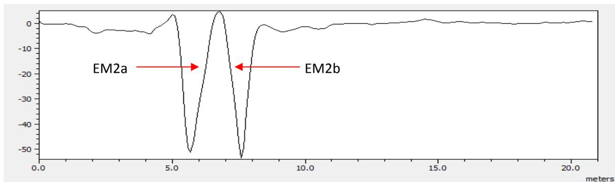
*Figure 45: Peak responses from EM2.a and EM2.b, displayed in a 2D magnetic profile. Profile alignment is delineated by the red dashed line in figure 44 from point A (0m) to point B (20m). Distance is expressed in meters on the bottom of the profile and readings are expressed in nT on the left hand side of the profile.*
