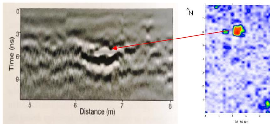
*Figure 10 (left): a two dimensional profile containing a Hohokam horno (earth oven) note individual heating elements cannot be seen, however the baked base layer can be easily seen.*
