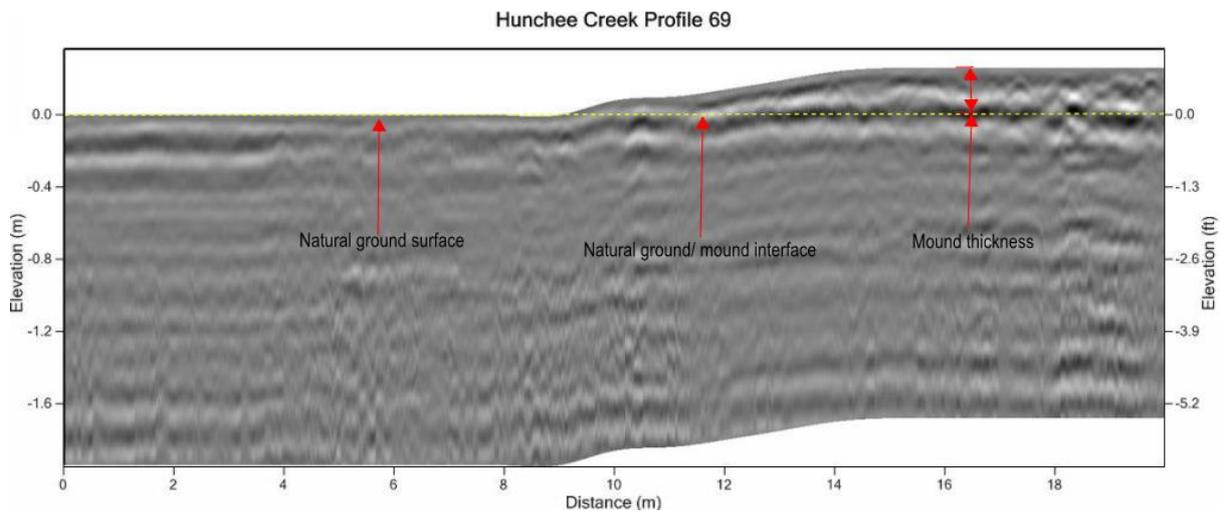
Figure 60: 2D GPR profile 69 topographically corrected and annotated, mound extents and depth were derived from all other profiles in this manner.
