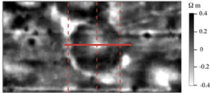
Figure 8: Resistivity survey over a hearth, the intersection of the solid line and middle dashed line delineates the centre of the hearth, the feature is circular in shape, note the subtle responses from the feature (plan view of dataset). The amplitude bar scale relates directly to the dataset and is expressed in Ohms (From Matney 2014:319).
