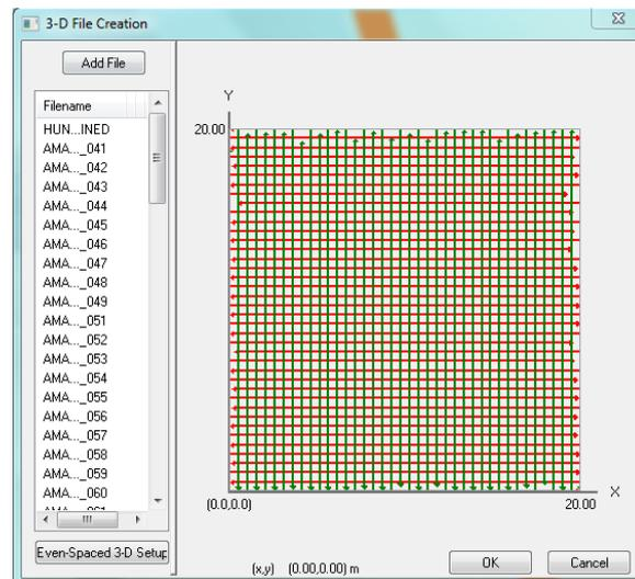
*Figure 55: survey configuration conducted over grid seven, data was collected in a zig-zag configuration at 0.5m intervals totalling forty scans acquired in each orientation.*
