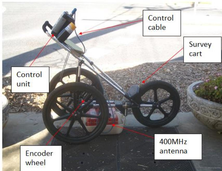
*Figure 22: A Geographical Survey Systems Inc. (GSSI) Ground Penetrating Radar System used on this project.*
