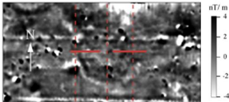
*Figure 7: Gradiometer dataset containing a hearth, cross hairs delineate the centre of the hearth which is circular in shape (this is a plan view of the dataset). The amplitude bar relates directly to the shades of the magnetics accompanying data set, readings are expressed in nano-tesla (From Matney 2014:319).*
