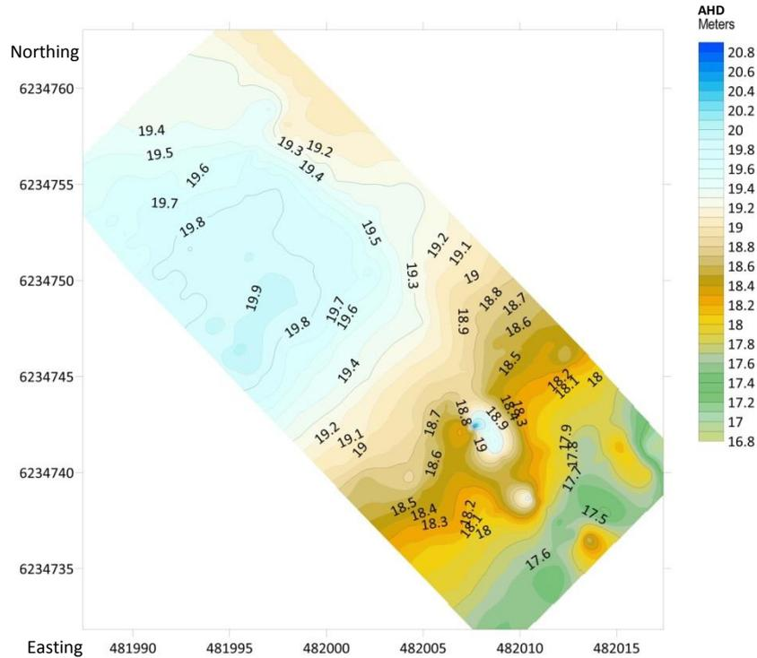
*Figure 67: Digital elevation model constructed from topographically surveyed electrode positions, EM2 is at the highest elevation of 19.9m with elevations gently sloping down to the river's edge at 17.5m at its lowest level.*
