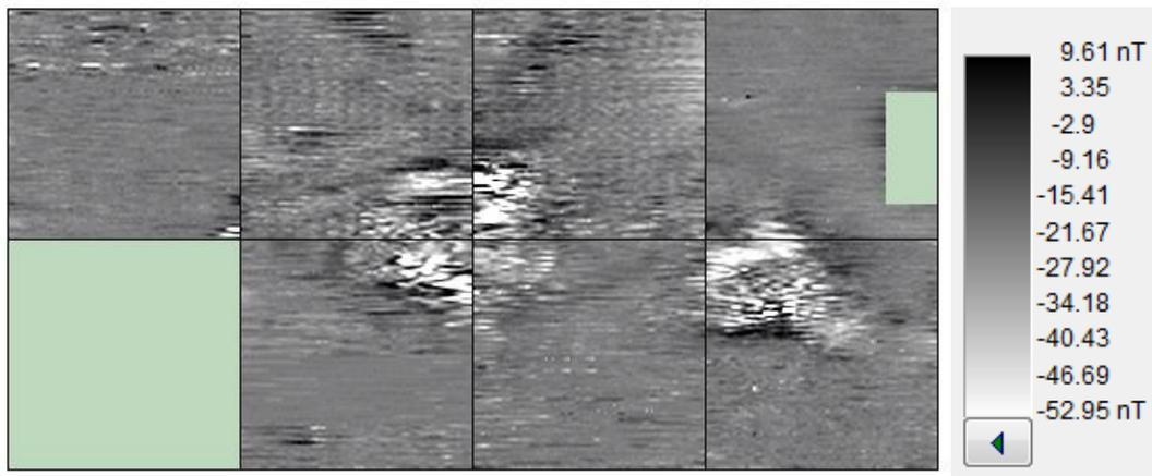
*Figure 29: The dataset after the 'mask' function has been applied, in the top right grid of the dataset the stormwater pipe has been removed resulting in other more subtle features becoming visible. Adjacent to the dataset is the colour scale of the data which is expressed in nano-tesla.*
