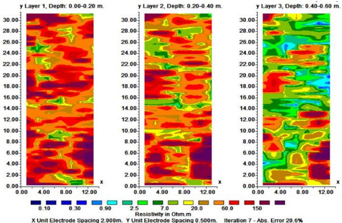
Figure 74: 3 Dipole-dipole array depth slices from the surface to 0.6m deep.
