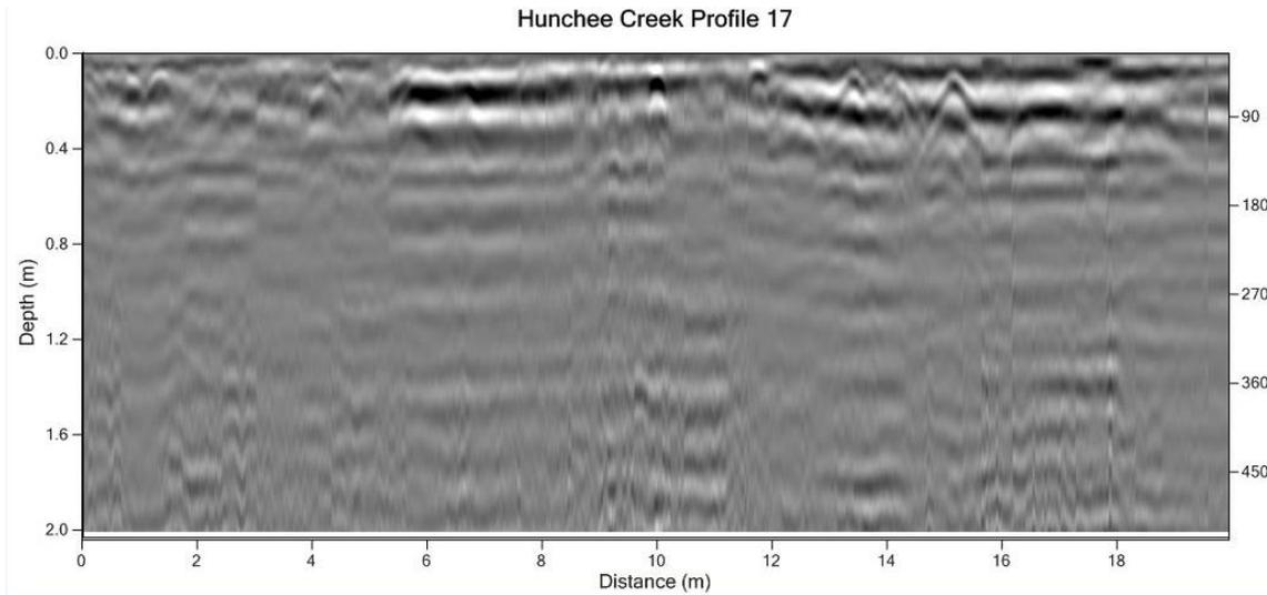
Figure 57: A 2D GPR profile 17 from the 3D dataset collected over grid seven, alignment depicted by the blue arrow in Figure 56, 0m is off the mound, the mound deposit starts at 10m and continues through to 20m.
