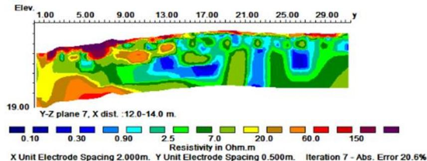
*Figure 30: An example of a pseudo-section after the inversion process, the data was collected over one of the earth mounds on this project. Readings are expressed in Ohms, colours in the pseudo-section correspond to the colour scale below, this data has been topographically corrected.*
