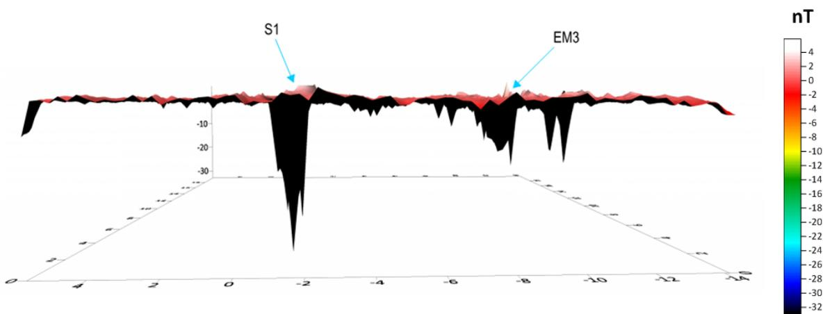
Figure 54: Side view of grid eight, the majority of magnetic readings are negative.
