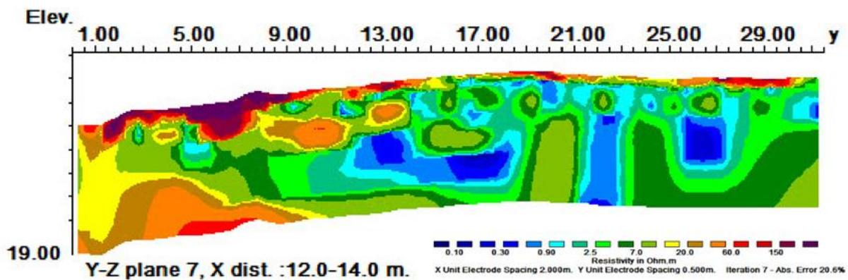
Figure 70: Dipole-dipole pseudo-section of the last electrode line of the survey, line 7.
