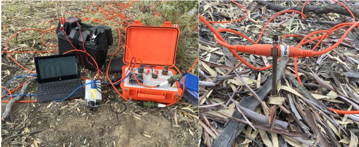
*Figure 23: The resistivity system used on this project (left) and one of 64 electrodes used to transmit voltage into the ground (right).*
