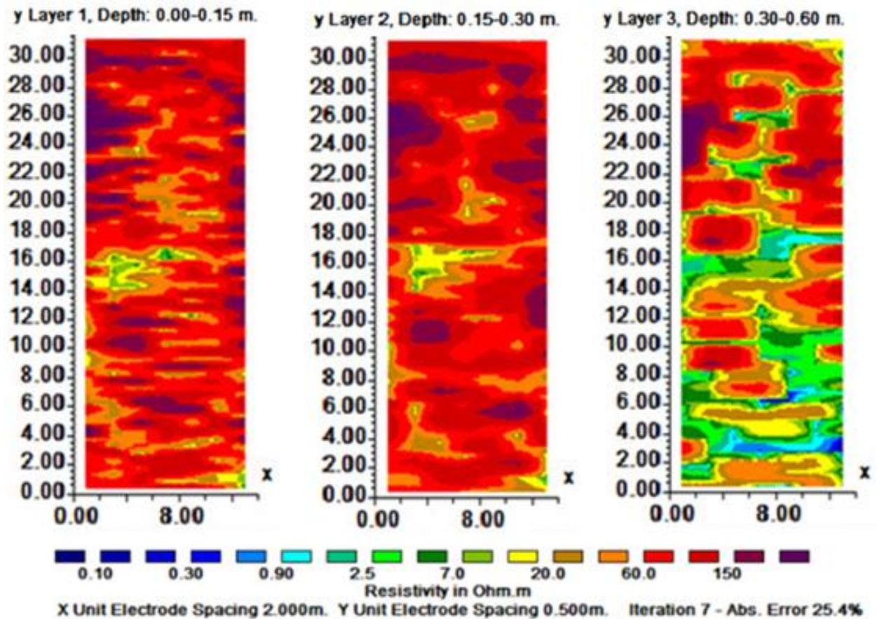
Figure 75: Three Wenner array depth slices from the surface to 0.6m deep.
