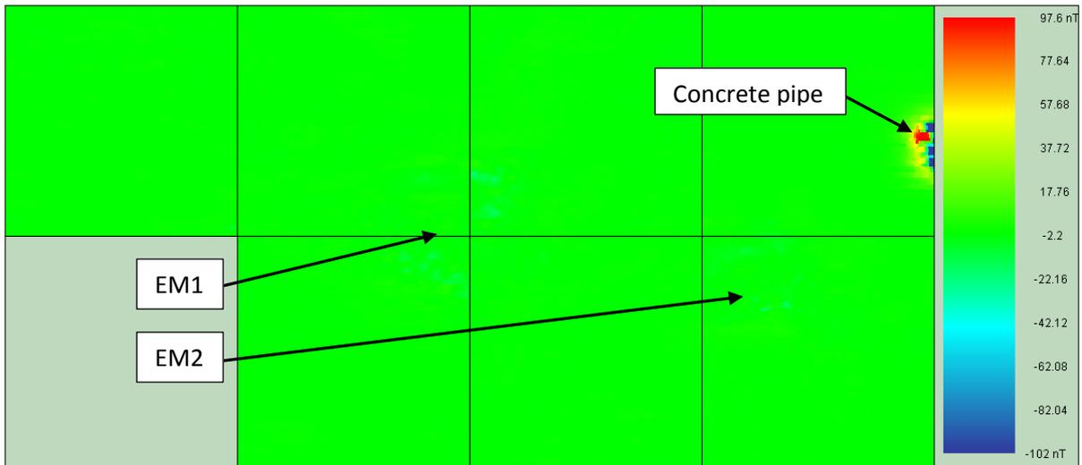
Figure 43: Grids one to seven – the high readings of the concrete pipe running under the road have resulted in EM1 and EM2 becoming virtually invisible, therefore the pipe needed to be eliminated from the dataset.
