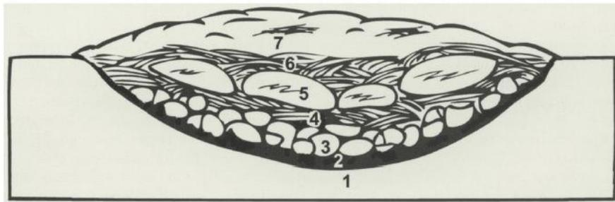
Figure 5: a cross section of an earth oven, from Black and Thoms (2014:205) as can be seen the earth oven diagram shows 7 layers. 1.prepared surface(oven pit), 2. Fire (reduced to ashes and glowing coals by the time the oven is sealed), 3. Layer of red-hot rocks (heating element), 4. Lower layer of green plant material (packing), 5. Food layer, 6. Upper layer of packing, and 7. Earthen cap.
