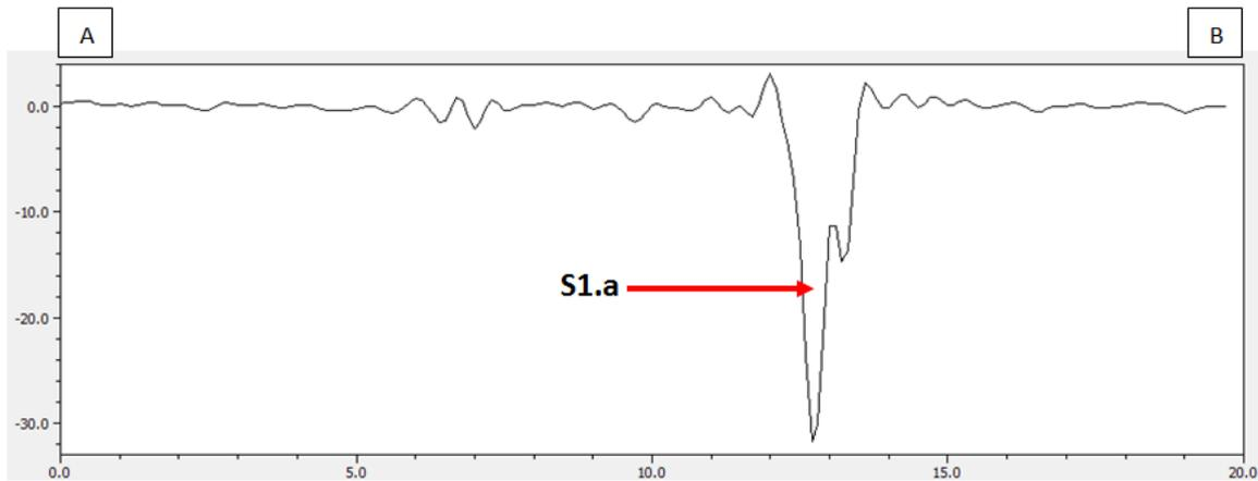
Figure 51: Peak response from a partially exposed earth oven composed of clay. Profile alignment is delineated by the red line from point A (0m) to point B (20m). Distance is expressed in meters on the bottom of the profile and readings are expressed in nT on the left hand side of the profile.
