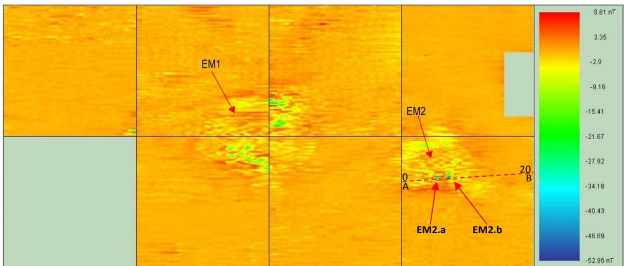
Figure 44: The main magnetics survey grid data set, grids one to seven are 20m x 20m grids collected with 0.25m line spacing. The scale of readings in nano-tesla to the right of the main survey grid corresponds to the colour of the readings in the dataset.
