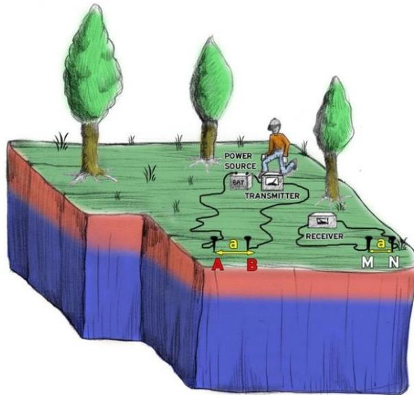
*Figure 25: dipole-dipole array survey configuration,  $a$  = electrode spacing,  $A + B$  = current electrodes,  $M + N$  = potential electrodes. The distance between the current electrode 'A' and 'B' (current dipole) and the distance between the potential electrodes 'M' and 'N' (measuring dipole) information from different depths is obtained by changing the distance from  $A+B$  and  $M+N$  from one another along the electrode line (diagram created by Kleanthis Simyrdanis).*
