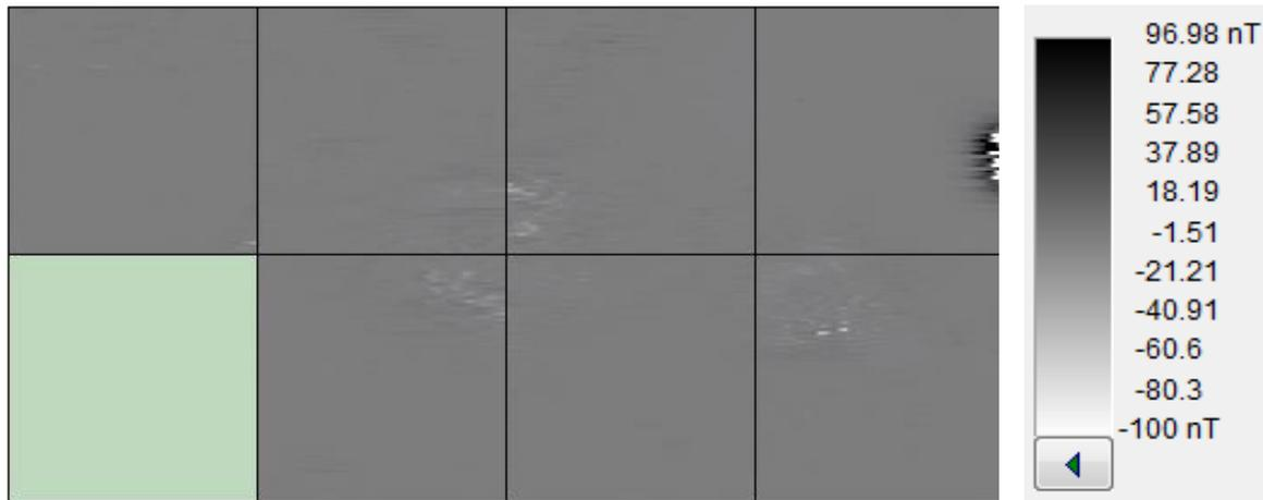
*Figure 28: Magnetics dataset after the 'destripe' function has been applied. Responses from the concrete pipe in the top right corner grid are masking more subtle responses.*
