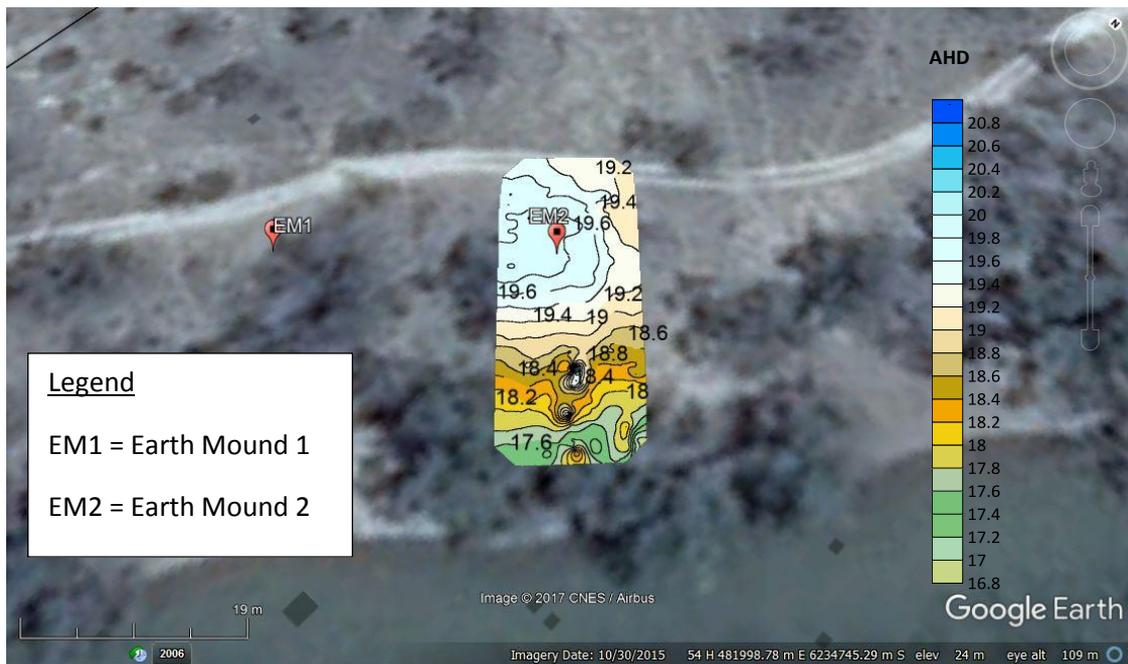
Figure 66: Digital elevation model constructed from topographically surveyed electrode positions, survey was located within grid seven – photo courtesy of google earth.
