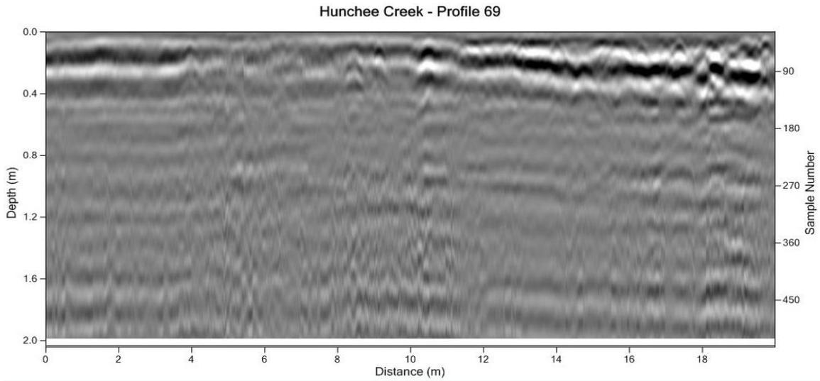
Figure 59: A 2D GPR profile from the 3D dataset collected over grid seven, alignment depicted by the green arrow in Figure 56, 0m is off the mound, the mound deposit starts at 11m and continues through to 20m.
