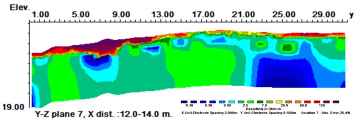
Figure 73: Wenner Array pseudo-section electrode line 7, the last line collected of the survey grid.
