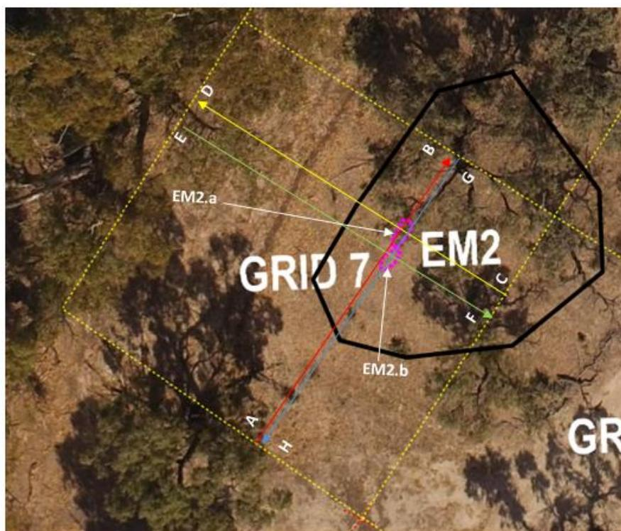
Figure 61: Combined GPR and Magnetics profiles location and alignment map over grid seven.
