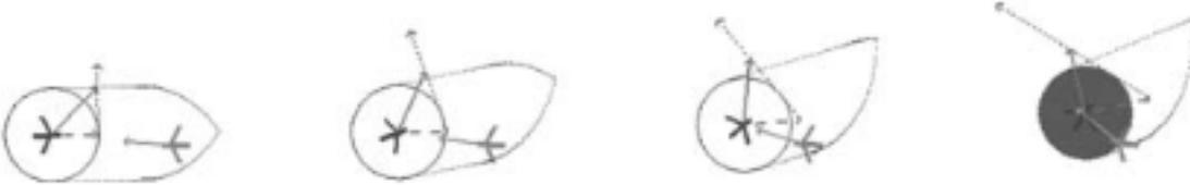
Figure 10: Pursuer starts within the reachable set, and thus can cause a collision despite the best efforts of the evader
