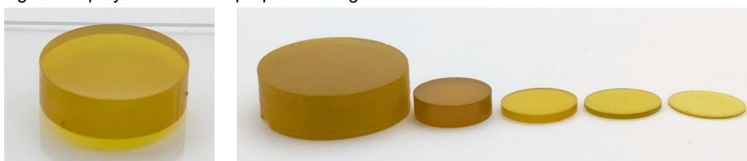
Figure 3.66: Images of polymer windows made from 81 % sulfur norbornane bistrisulfide polymer.
