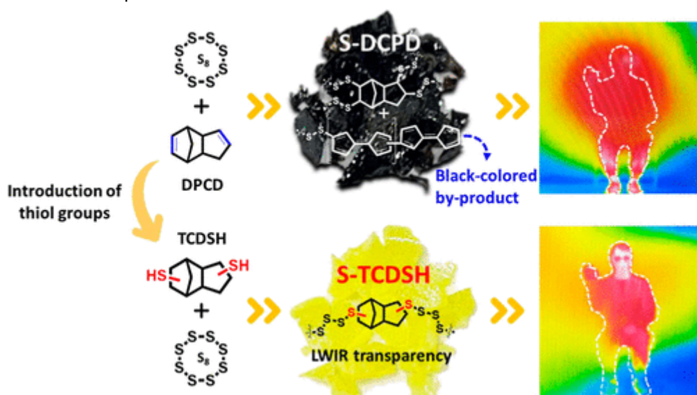
Figure 1.17: Introduction of thiol groups to dicyclopentadiene and inverse vulcanization to prepare long wave infrared transparent polymers. Reused with permission from. 129
