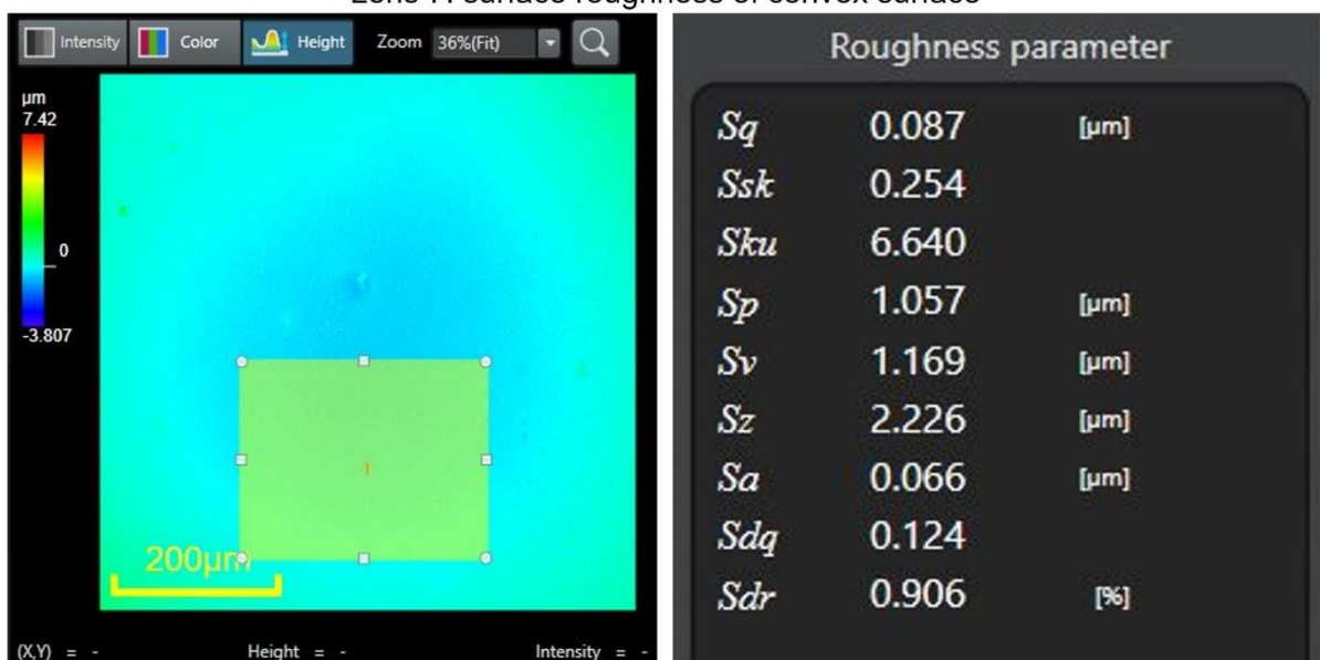
Lens 7: surface roughness of plano surface
