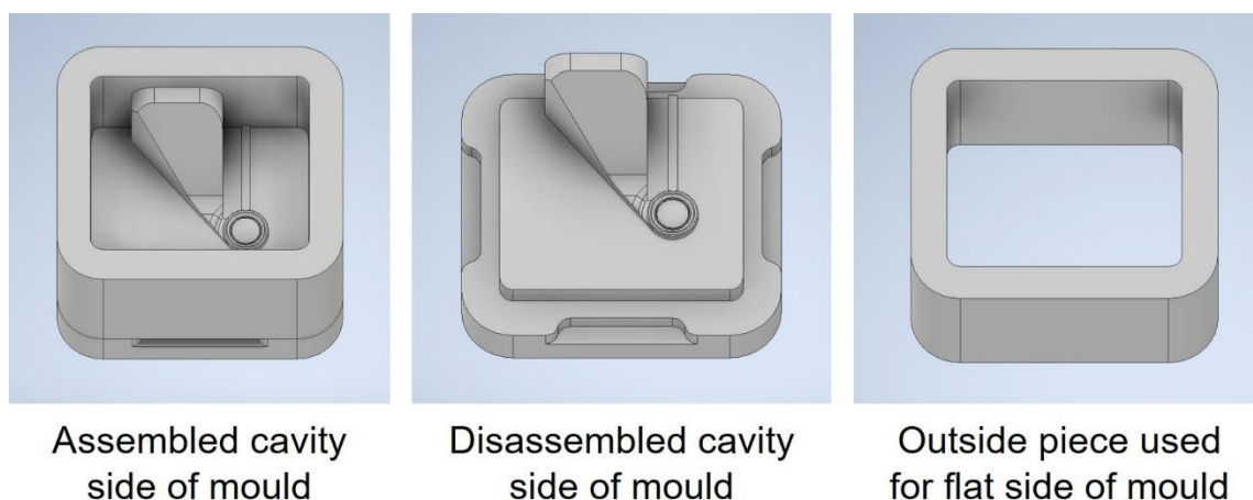
Figure 4.29: Design of two part mould in Autodesk Inventor.
