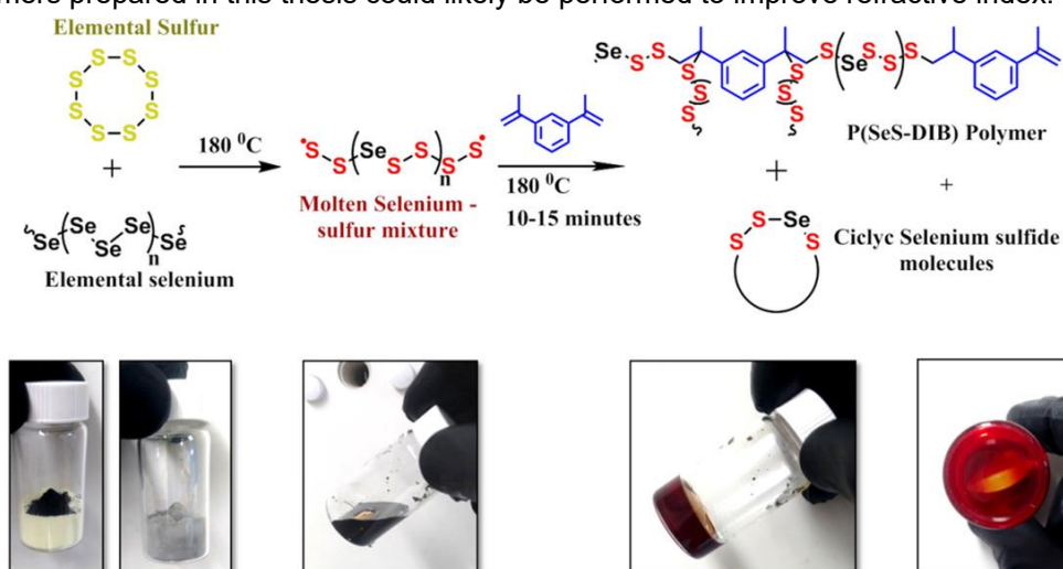
Figure 1.10: Process of incorporating selenium into polymers through inverse vulcanization to prepare high refractive index polymers. (structure likely incorrect due to corrected reaction mechanism). Reused with permission from. 117
