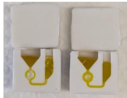
Path too long (no injection pressure)
