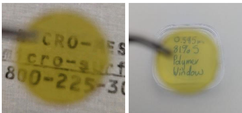
Figure 4. 25: Images of polymer window made from 81 % sulfur norbornane bistrisulfide polymer.
