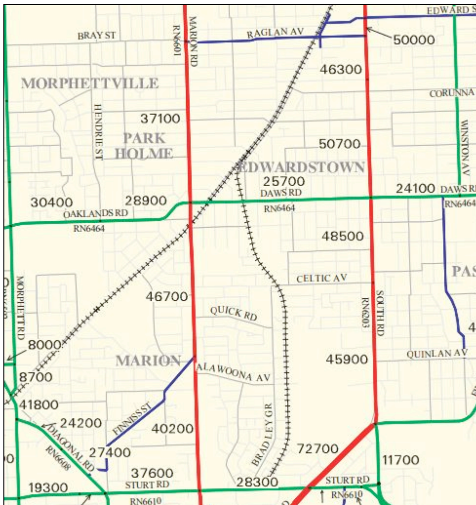
Figure 24. Road class and average traffic volumes of the two routes (DPTI, 2017).
