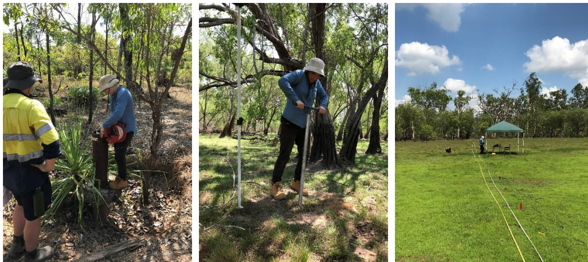
Figure 1.5. Field trips to Wildman River area. Collecting water level measurements (left), sediment samples (middle) and seismic refraction data (right).
