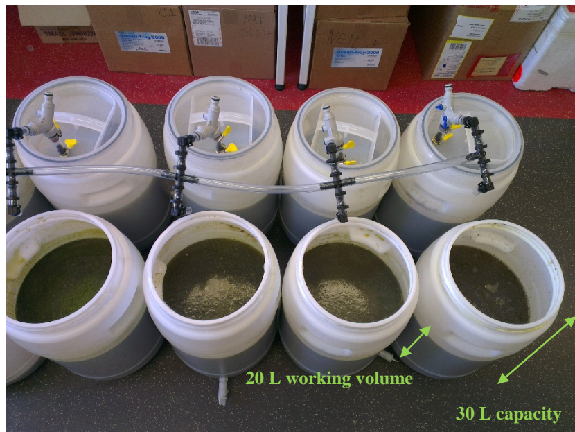
Fig. 4.4 The anaerobic digesters with different algal sludge (ALBAZOD)/pig slurry mixtures. The working volume was 20L.
