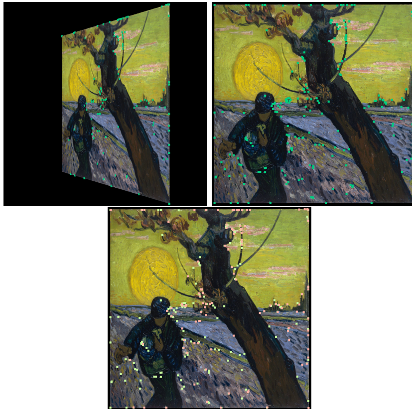
Figure 3.3: Y axis rotation with Foerstner detection of Sower image, with first image at -50^\circ , 0^\circ and both overlaid using matrix transforming of first image's interest points.
