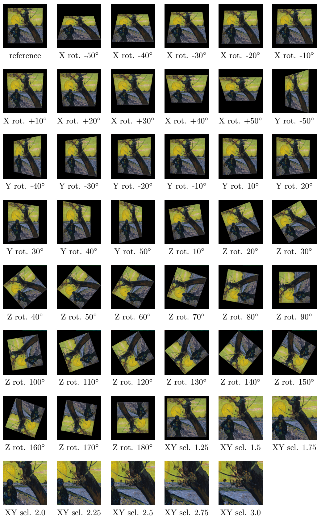
Figure A.5: Transforms used during evolutionary testing, consisting of X,Y and Z axis rotation and XY scaling. In this example the sower image is used.
