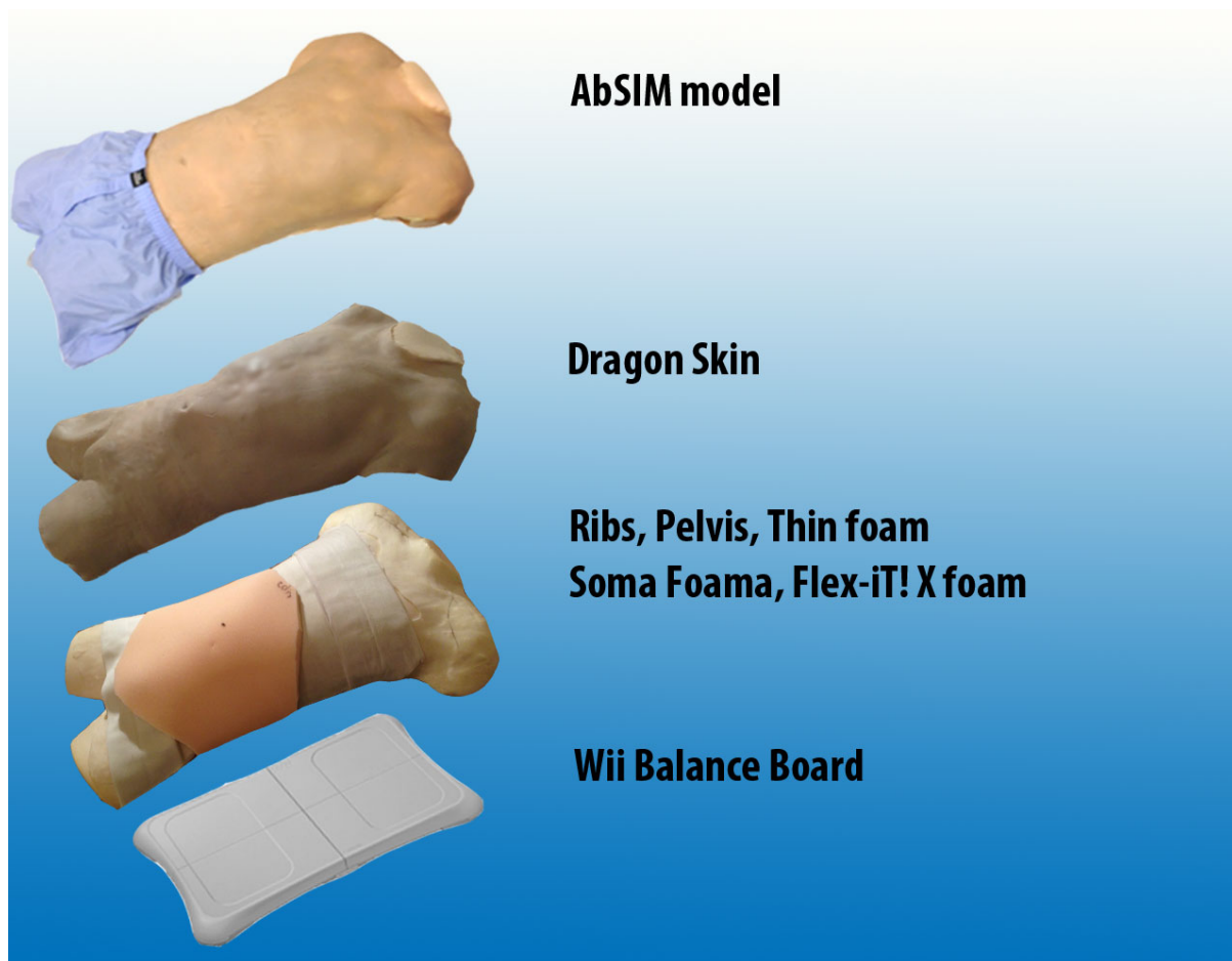
Figure 43. Exploded view of the various moulded layers in AbSIM
