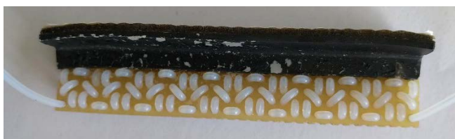
Figure 5-21. Woven heating coil tested for on-line conversion of cyclophosphamide
