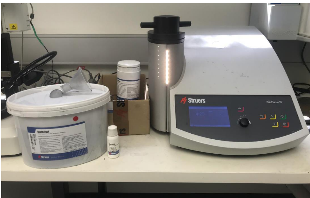
Fig. 4. Struers CitoPress-10 hot mounting press. Photograph by Wendy van Duivenvoorde.
