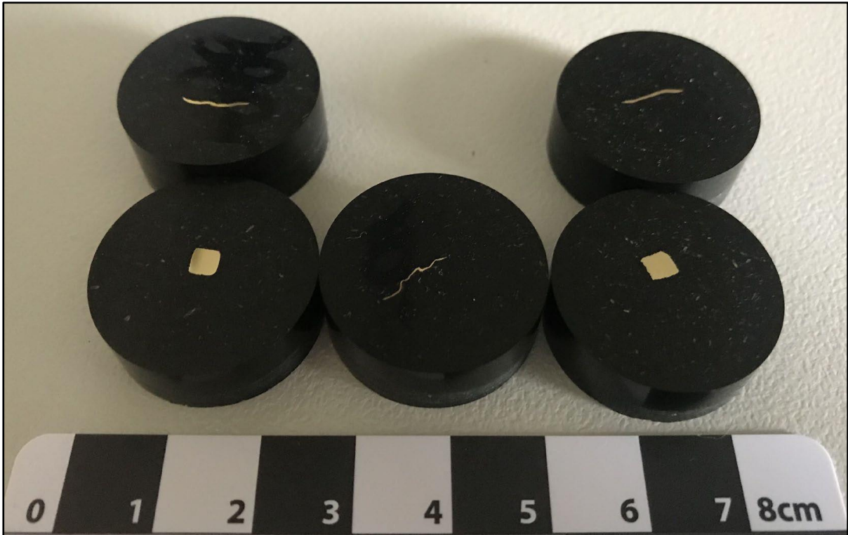
Figure 3.10. Examples of samples embedded in black-coloured resin, the top two samples and bottom centre are all metal sheathing whereas the bottom samples on left and right are cross sections of fasteners ( not South Australian shipwreck) (Photography by Wendy van Duivenvoorde)
