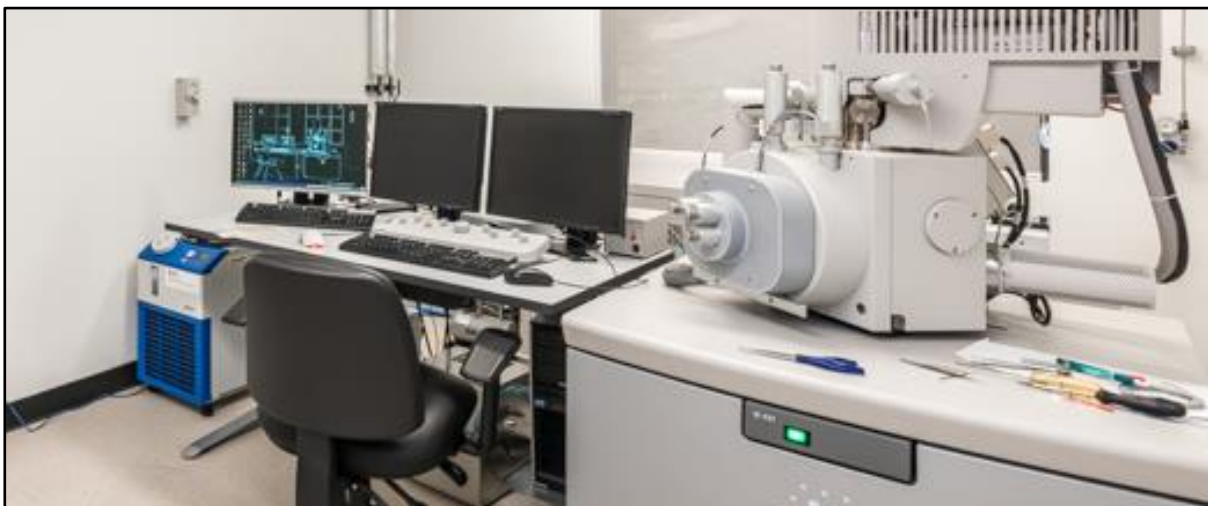
Figure 3.7. FEI Quanta 450 FEG Environmental Scanning Electron Microscope, Adelaide Microscopy, University of Adelaide (Photograph by Wendy van Duivenvoorde)
