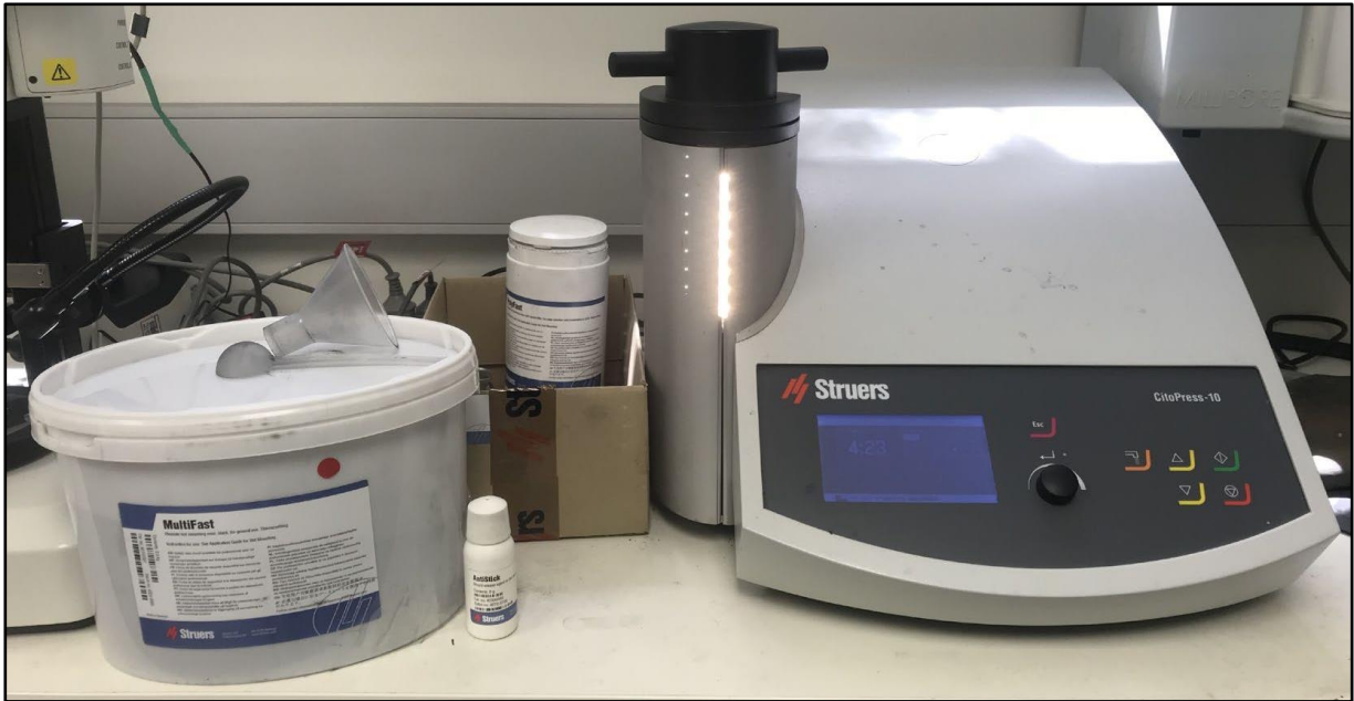
Figure 3.8. Struers CitoPress-10 hot mounting press (Photography by Wendy van Duivenvoorde)
