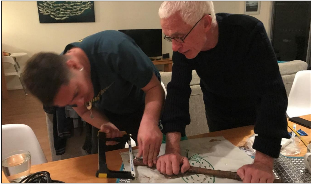
Figure 3.6. Timothy Zapor and Kieran Hosty extracting metal samples from a copper bolt (Photograph by Irimi Malliaros, June 23, 2019)
