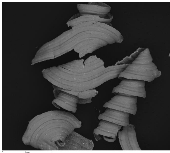
Fig. 8. Drill shavings of bolt (a) and magnified drill shaving showing spectrum analysed (b, Spectrum 1) ( South Australian shipwreck , keel pin 0404). White-coloured inclusions are lead.
