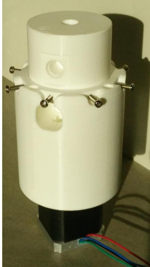
Figure 4.13: 3D Printed Valve and Motor Mounted to Assembly
