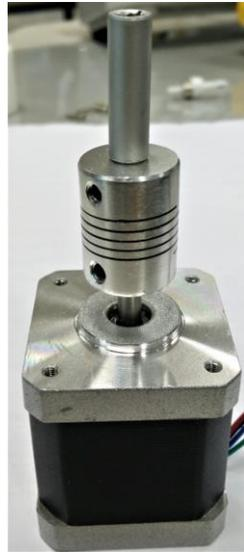
Figure 4.9: Stepper Motor and Shaft Assembly
