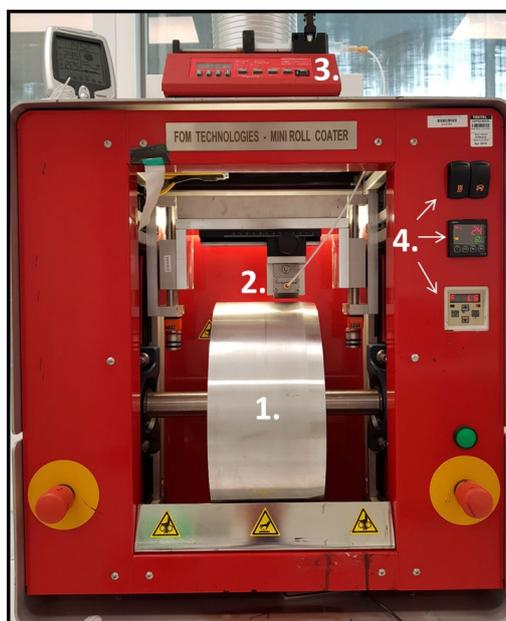
Figure 3.6: Mini-Roll coater for slot-die coating with 1) rotating/heated drum, 2) slot-die coating head, 3) syringe pump, and 4) rotation and temperature controls. In operation, a flexible substrate is attached to the rotating drum and the slot-die coating head is lowered to allow formation of a meniscus between substrate and head.
