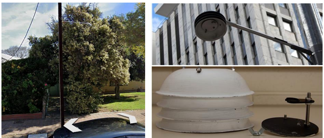
Figure 2. 5 Photographs showing how a radiation shield is installed on a light pole (left). Bottom view and major components of a radiation shield (right).
