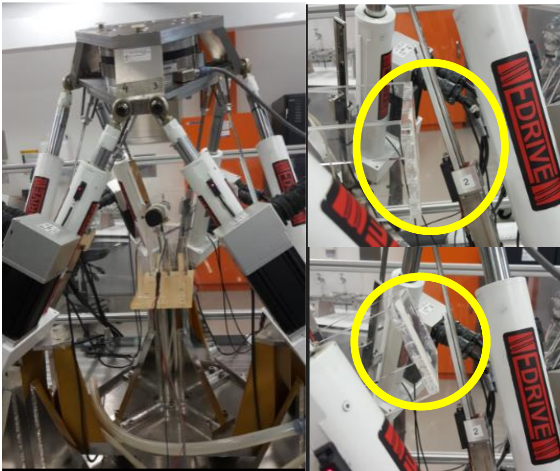
Figure 2.18. The yellow circles indicate the position of the cradle and encoder. Hexapod in R_x = -20^\circ (left) with cradle at 90° (right top) and 120° (right bottom) at a physical distance of 21 mm.
