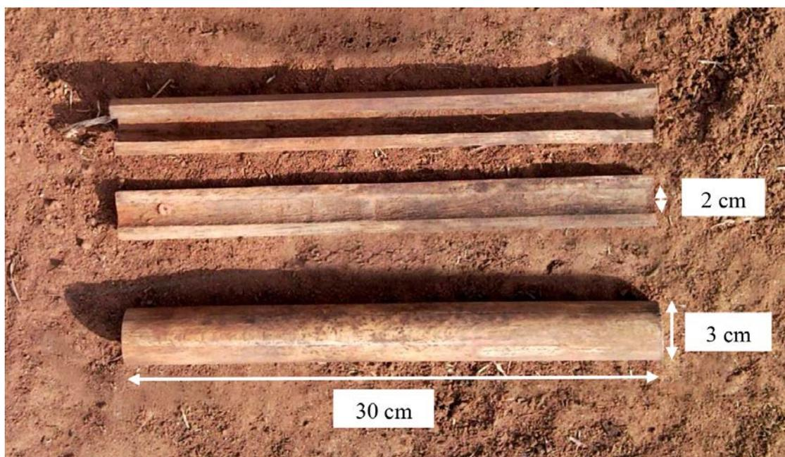
Figure 2-6. Wooden dowling artificial burrows. The upper two images are the two halves of a burrow that has been cut open to reveal the internal structure.
