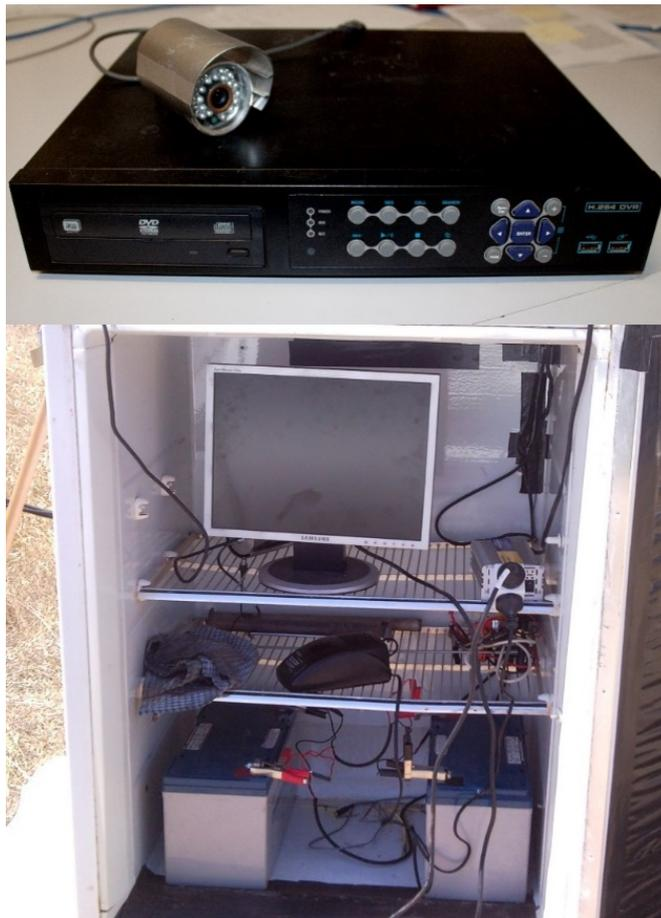
Figure 2-10. DVR, cameras and batteries we used for filming lizard behaviour
