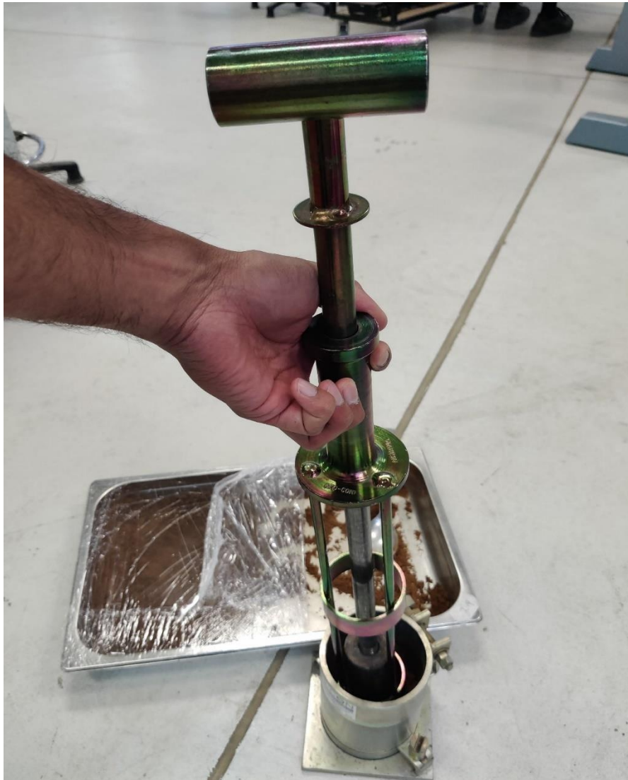
Figure 11: Soil with 1% Add Plastic Strips with Compaction Test
