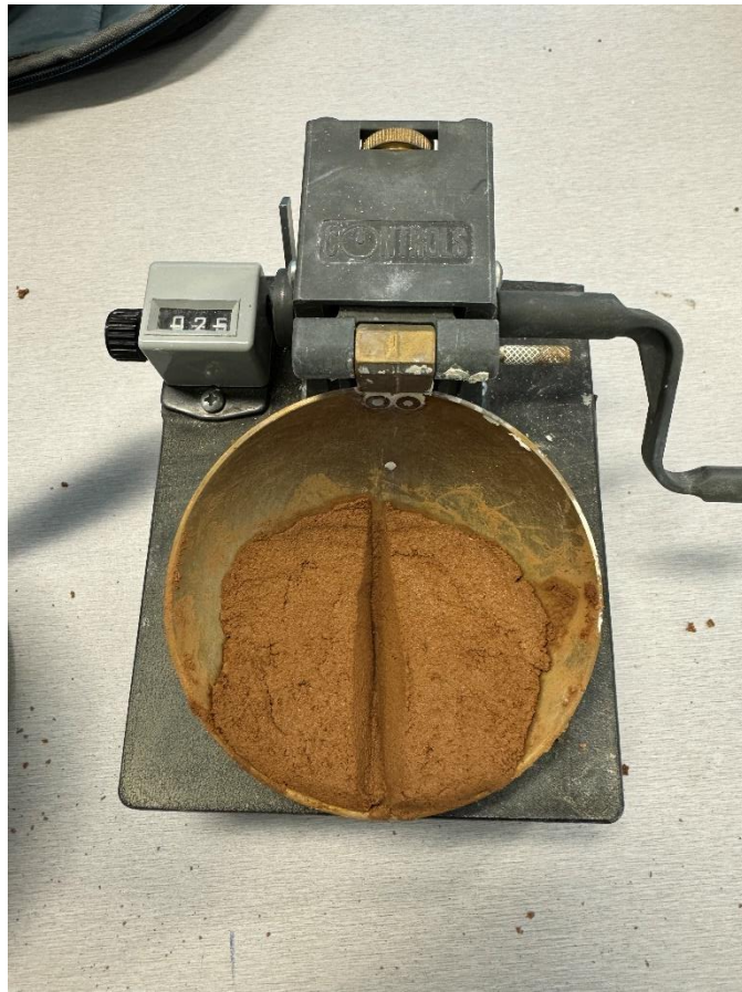
Figure 13: Liquid Limit Cup Method
