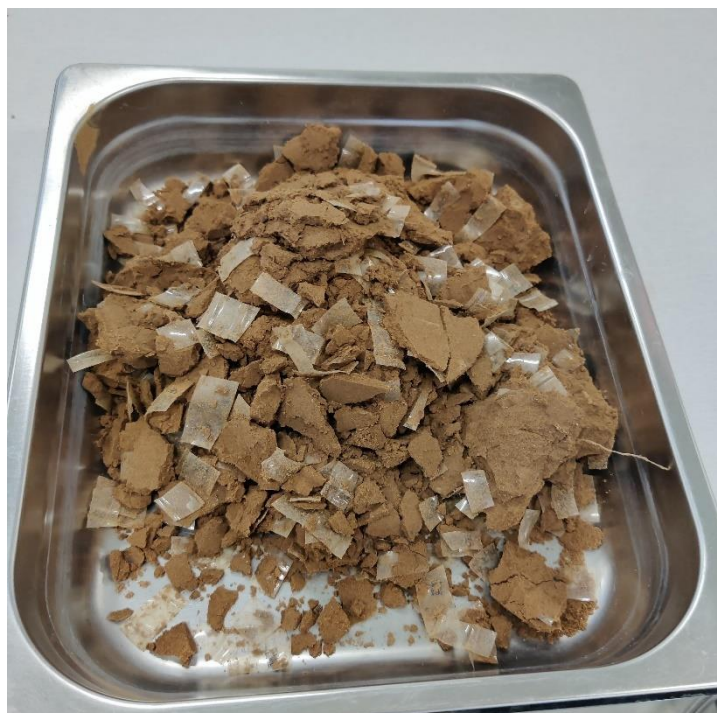
Figure 12: Failure of 1 st Sample in Compaction Test
