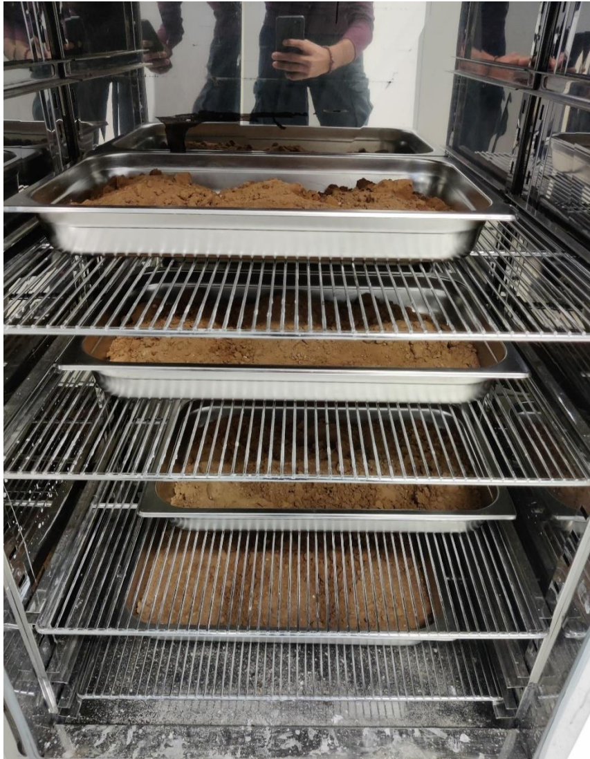
Figure 9: Soil Samples Drying in an Oven
