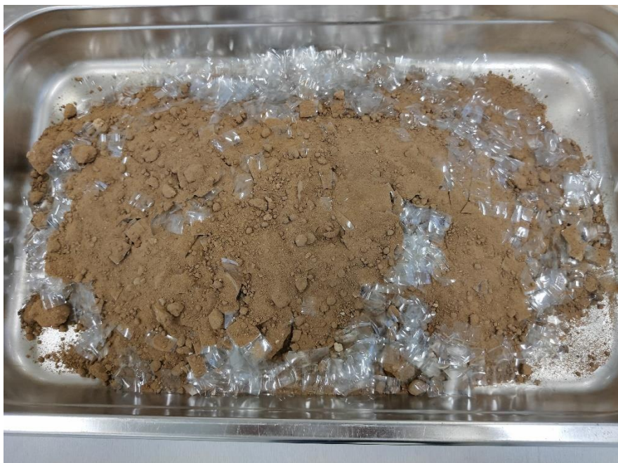
Figure 10: Clay Soil Samples with Admixture Plastic Strips
