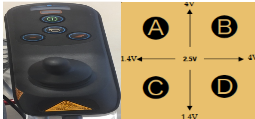
Figure 7. Joystick on wheelchair and voltage output range from joystick
