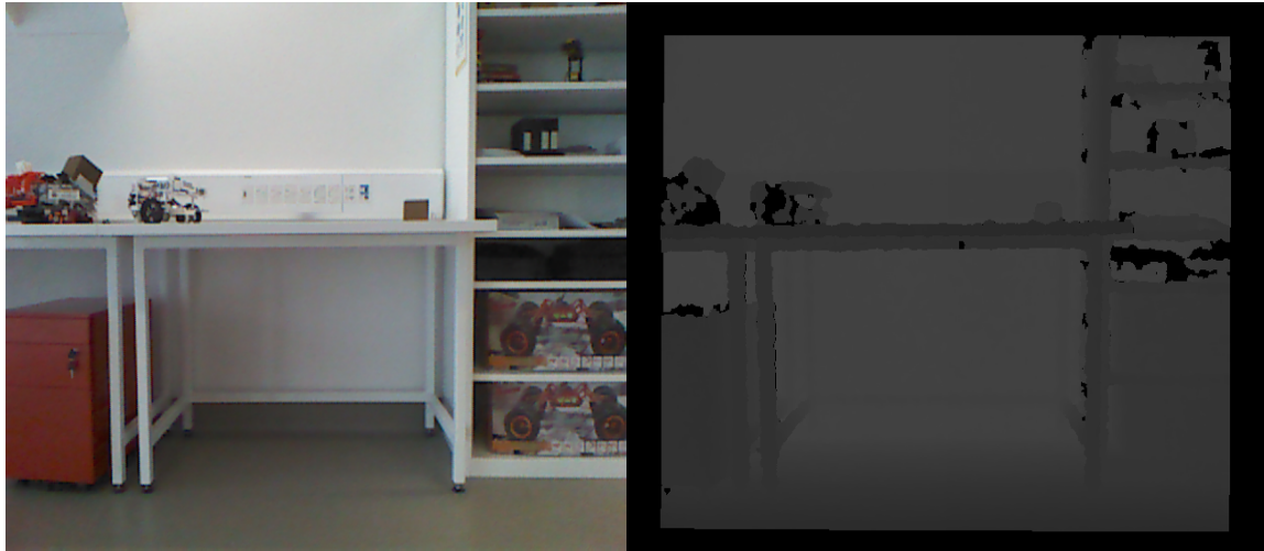
Figure 53. RGB image and depth image from the Kinect sensor
