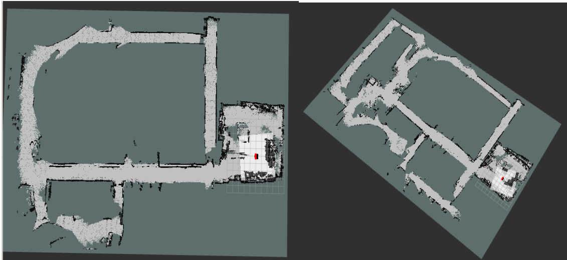
Figure 60. Grid maps generated from depth image for stages 1 and 2
