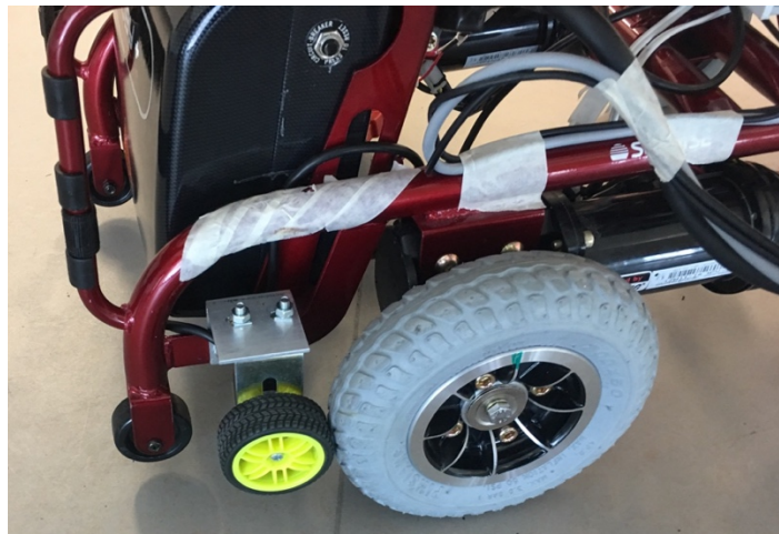
Figure 22. Wheel on wheel configuration for encoders
