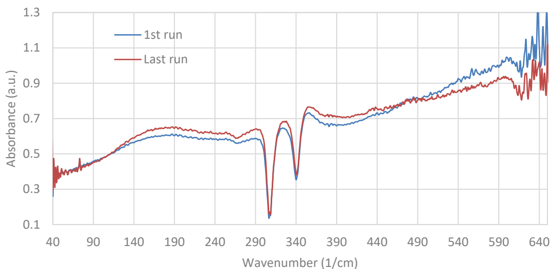
Figure 1-79: Overlaid absorbance spectra of incubated (40 degrees water bath) bilirubin in DMSO-d6 (4 mg in 25 \mu L DMSO-d6) in DWLC C using 20 \mu m spacer, analysed overnight at the Australian Synchrotron (FIR Beamline) with SiBolo detector. Amplitude 5380.
