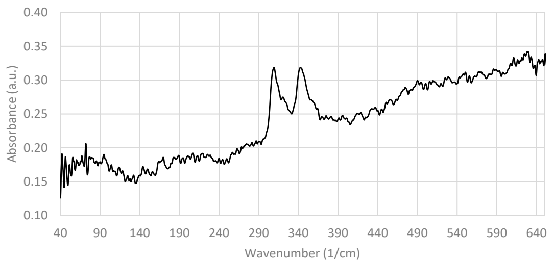
Figure 1-38: FIR spectrum of DMSO-d6 in DWLC A with a 10 \mu\text{m} spacer, analysed at the Australian Synchrotron (FIR Beamline) with SiBolo detector. Amplitude 6090.
