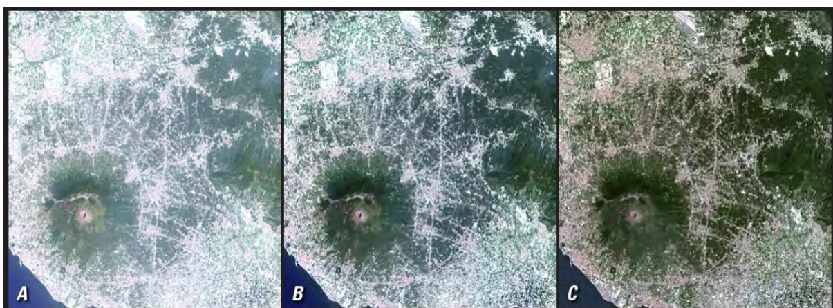
Figure 8: Subsets of a Landsat scene of Mount Vesuvius near Naples, Italy, display A, natural color composite; B, top-of-atmosphere reflectance and C, surface reflectance processing
