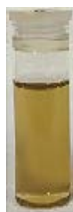
Figure 3-3. Photograph of FL-BP in NMP prepared by exfoliating bulk BP using ultrasonication for 24 h.
